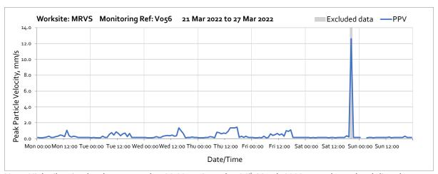
Note: High vibration levels measured at 20:00 on Saturday 26<sup>th</sup> March 2022 were due to local disturbance at the monitoring location and not representative of HS2 vibration levels at the receptor. Missing data in between 01:00 and 02:00 on Sunday 27<sup>th</sup> March was due to the clocks going forward at the start of British Summer Time.
