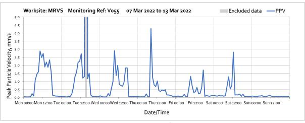
Note: High vibration levels measured at 15:00 on Tuesday 8<sup>th</sup> March 2022 were due to local disturbance at the monitoring location and not representative of HS2 vibration levels at the receptor.
