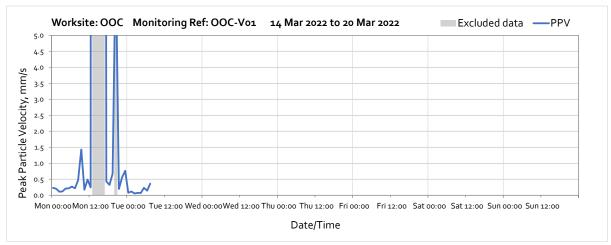
Note: High vibration levels measured across the week were due to local disturbance at the monitoring location and not representative of HS2 vibration levels at the receptor. The monitor has been removed from site on Tuesday 15<sup>th</sup> March 2022.
