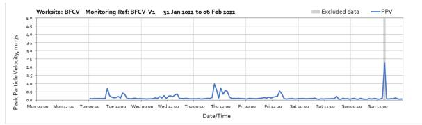
Note: High vibration levels recorded at 15:00 on 6<sup>th</sup> February were due to local disturbance at the monitor location and therefore not representative of HS2 vibration levels at the receptor.
