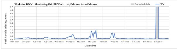
Note: High vibration levels recorded at 10:00 on Saturday 20<sup>th</sup> February were due to local disturbance at the monitor location and therefore not representative of HS2 vibration levels at the receptor .
