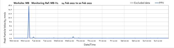
Note: High vibration levels recorded at 16:00 on 14<sup>th</sup> February was due to HS2 related drainage, setup of piling mats and stockpiling works undertaken at close proximity to the vibration monitor.
