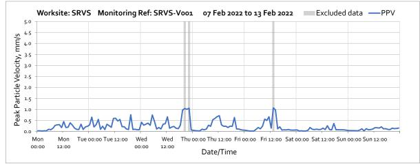
Note: High vibration levels measured throughout the week are due to local interference and not representative of HS2 vibration levels at the receptor.
