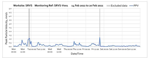
Note: High vibration levels measured throughout the week are due to local interference and not representative of HS2 vibration levels at the receptor.
