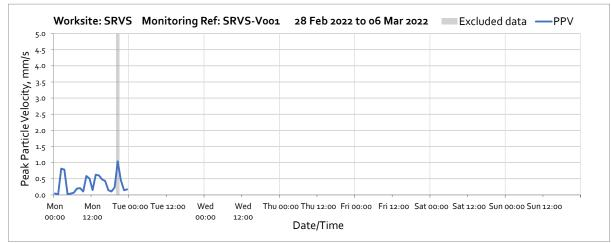
Note: High vibration levels measured at 20:00 on Monday 28<sup>th</sup> February are due to local interference and not representative of HS2 vibration levels at the receptor.
