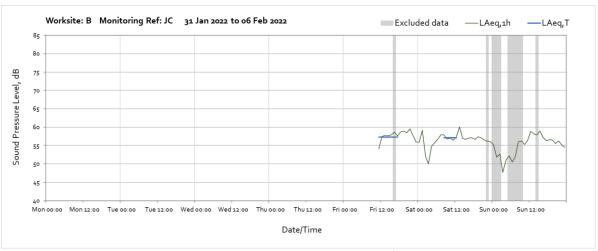
Note: Missing data from the start of the month until 11:00 on Friday 4<sup>th</sup> February was due to loss of power to the monitoring station caused by a damaged power supply unit. The power supply unit has been repaired with view of minimising loss of data in the future.
