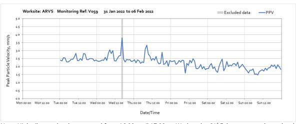
Note: High vibraton levels measured from 16:00 until 17:00 on Wednesday 2<sup>nd</sup> February were due to local interference of the monitor and are not representative of HS2 vibration levels at the receptor.
