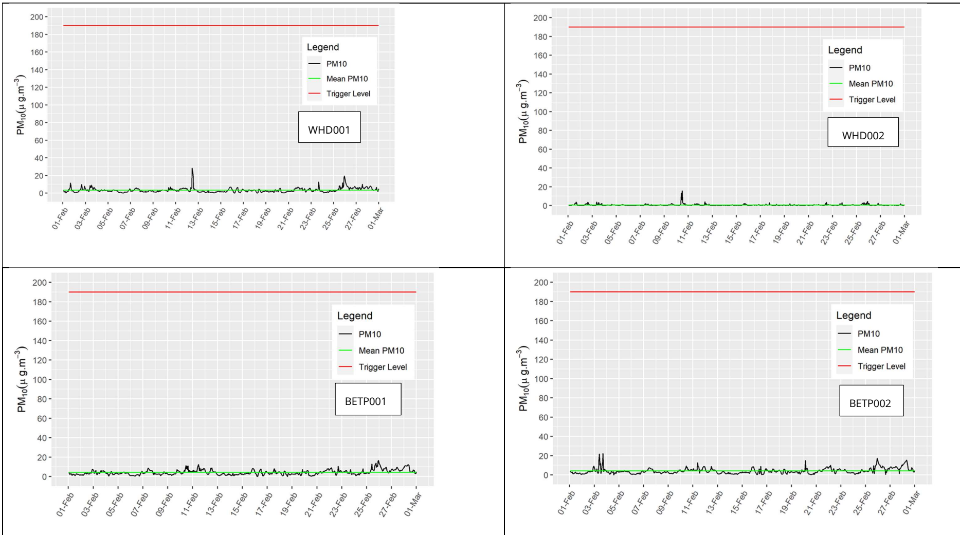
Figure 23: Construction dust 1-hour mean indicative PM 10 concentration for all dust monitors
