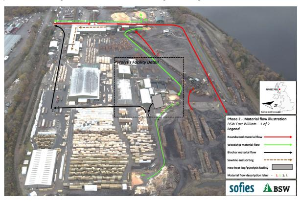
Figure 8 - Material flow diagram of the Fort William sawmill with biochar production
