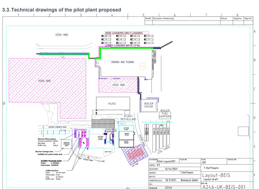
Figure 5 – Technical drawing displaying proposed Biomacon pyrolysis facility (labelled in bottom left) integrated with upgraded BSW "hotties" heatlog production line. Flecible biochar production facility comprises of two biomacon c-500l units and accompanying moving floor feed intake systems and extraction/packing systems.
