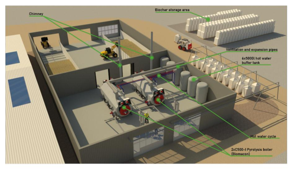
Figure 6 – 3D rendered visulisation of two side by side Biomacon C500l units at BSW Fort William. Heat will be transferred from hot water buffer tanks to BSW heat sinks (both in woodchip and timber drying processes).
