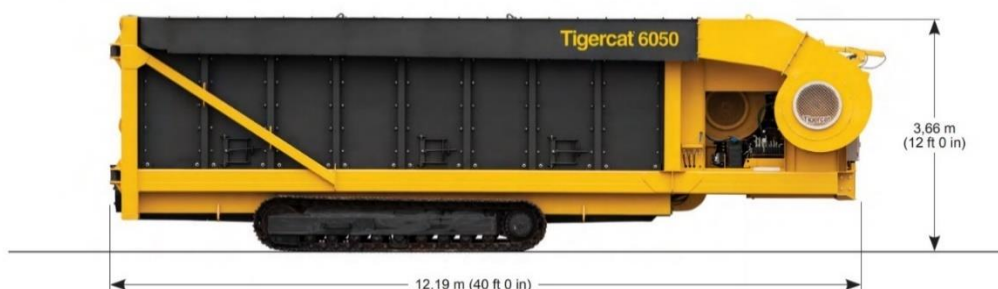
Figure 15: Annotated picture to show dimensions of Tigercat 6050 Carbonator (Tigercat, 2021)
