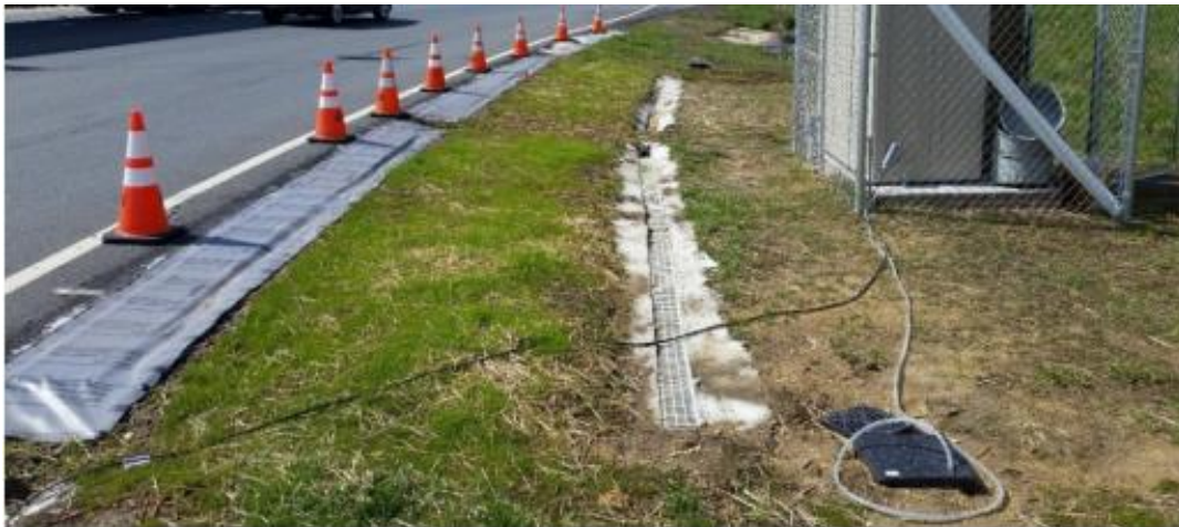
Figure 2: Photo to show biochar amended verge (Imhoff & Nakhli, Reducing Stormwater Runoff and Pollutant Loading with Biochar Addition to Highway Greenways , 2017)
