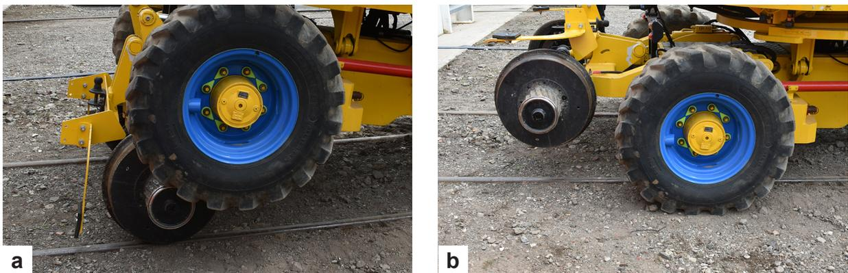
Figure 4: MEWP rail axle configurations in (a) rail configuration and (b) road configuration
