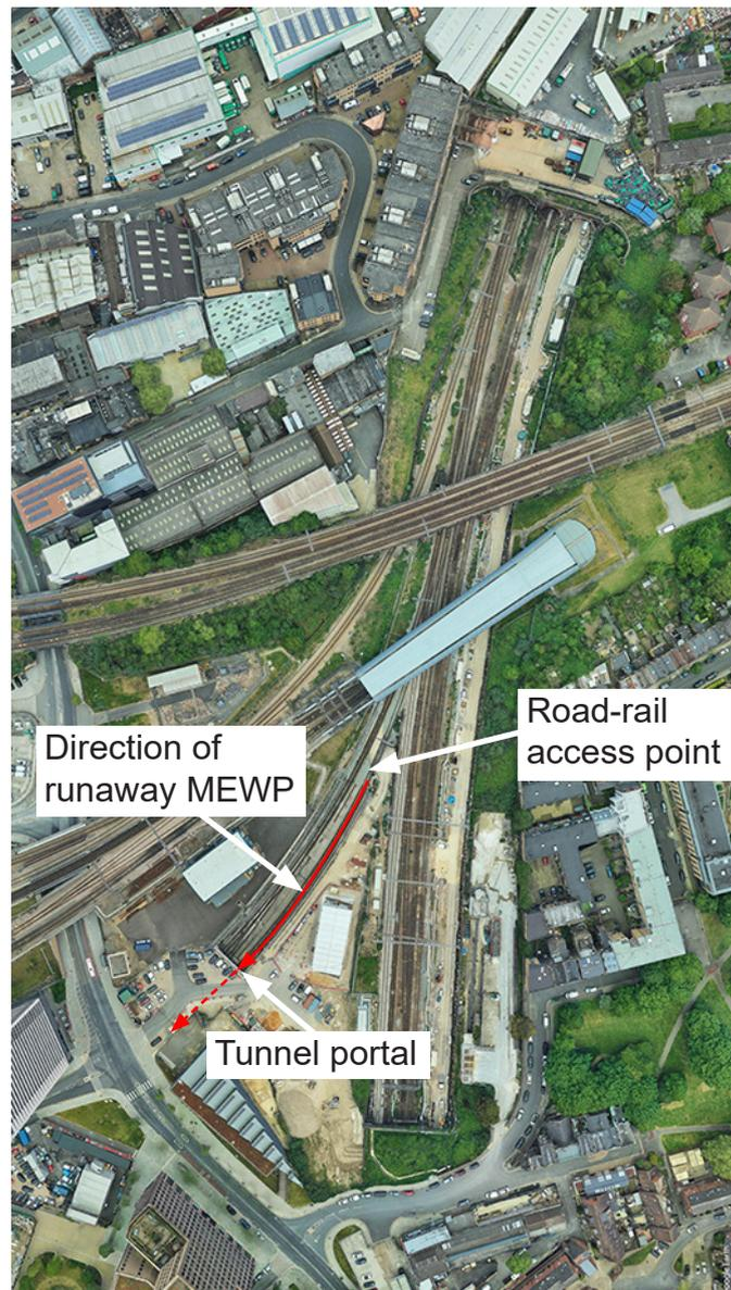
Figure 2: Overview of RRAP showing geographical relationship of key features and the path taken by the MEWP
