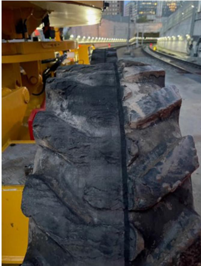
Figure 8: Road tyre wear profile
