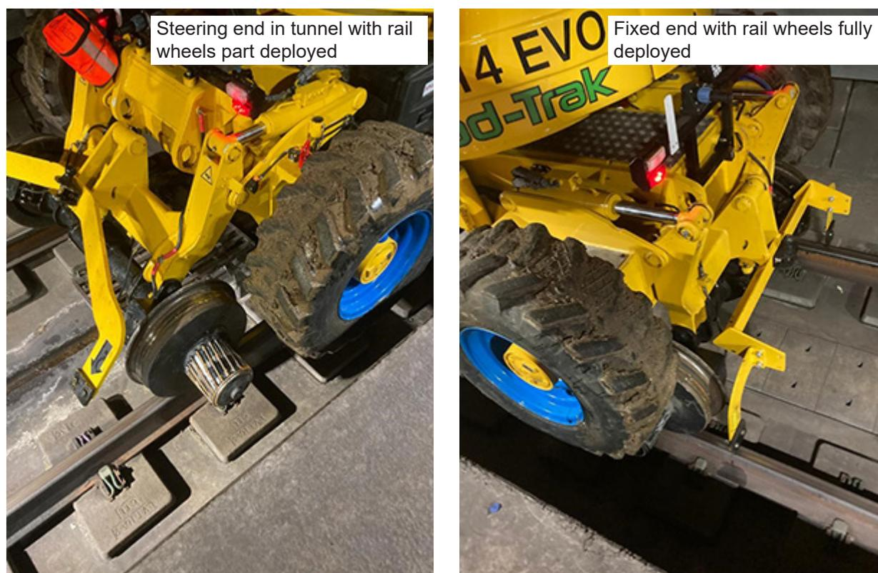
Figure 5: The position of the rail axles when the MEWP came to rest (images courtesy of Network Rail)
