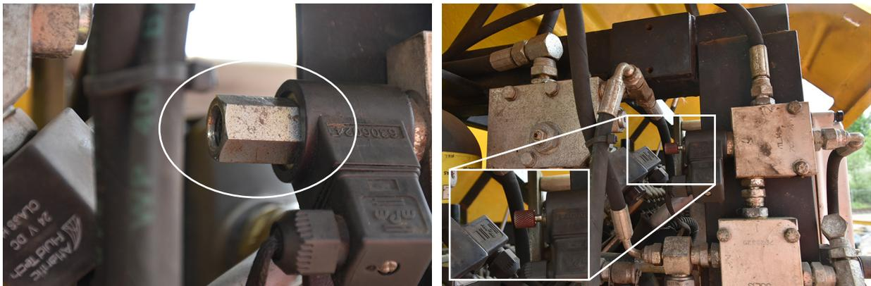
Figure 7: the park brake valve with barrel nut fitted (left) and removed, exposing the knurled knob (right)
