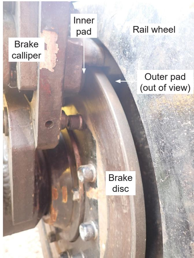
Figure 6: DRWB calliper and disc arrangement
