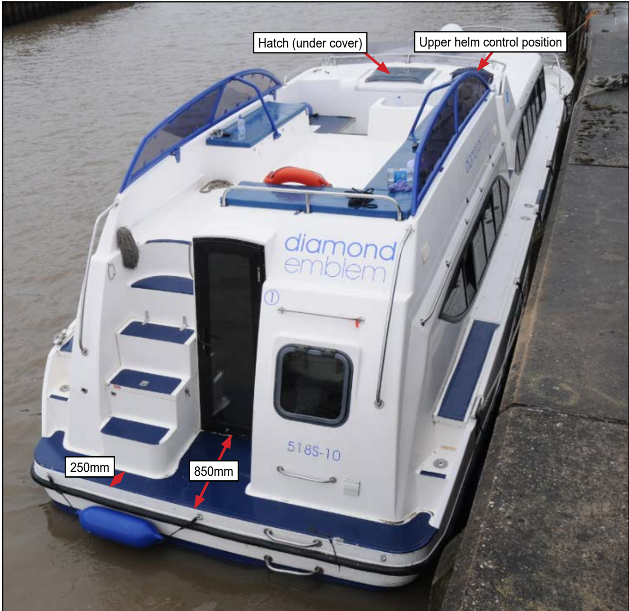
Figure 10: Aft deck and staircase between upper and lower decks on Diamond Emblem 1
