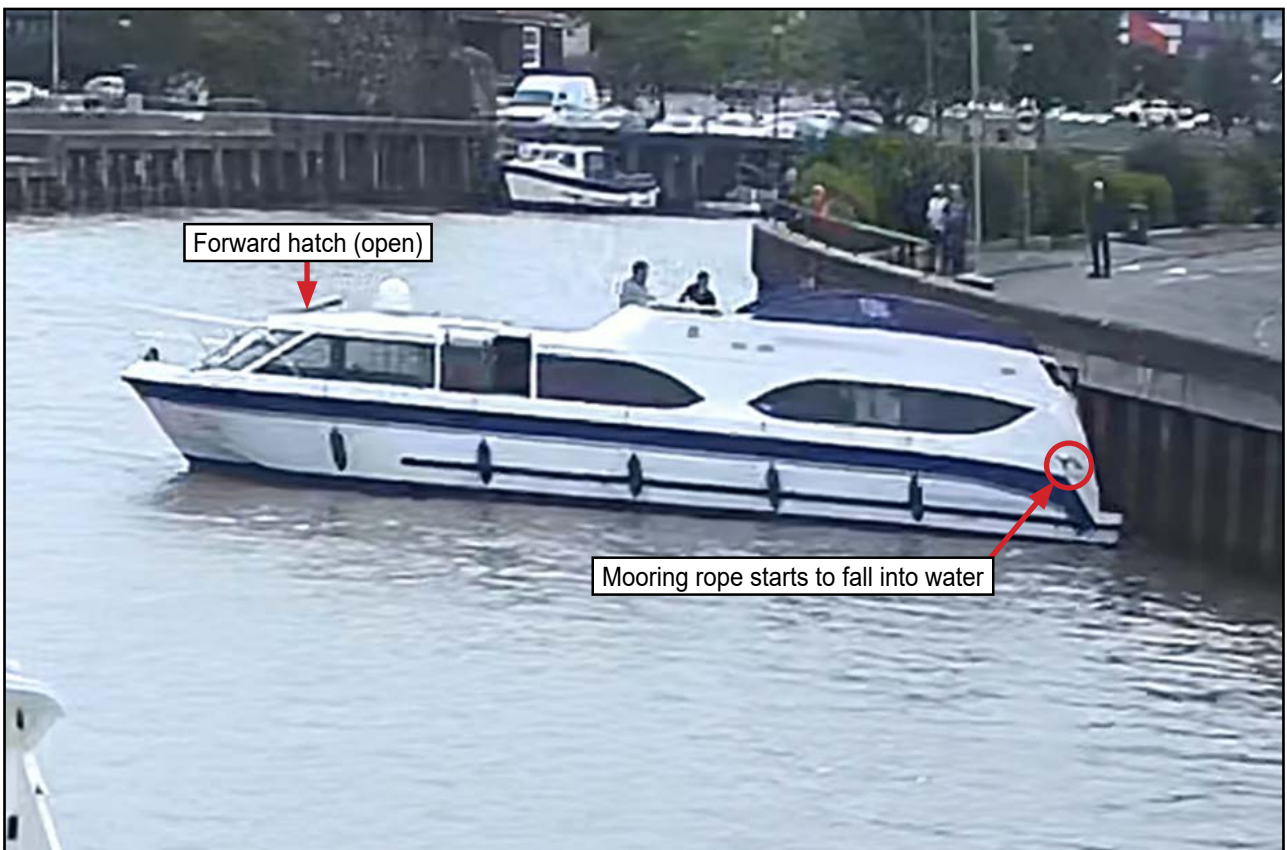
Figure 8b: Mooring rope on port aft deck of Diamond Emblem 1 falling into the water at 1318:01
