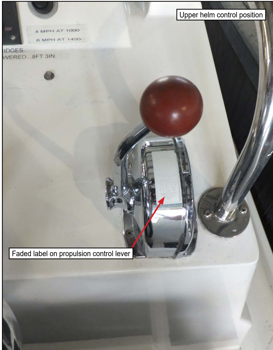
Figure 14: Faded propulsion control labelling at upper and lower helm control positions at time of Diamond Emblem 1 accident
