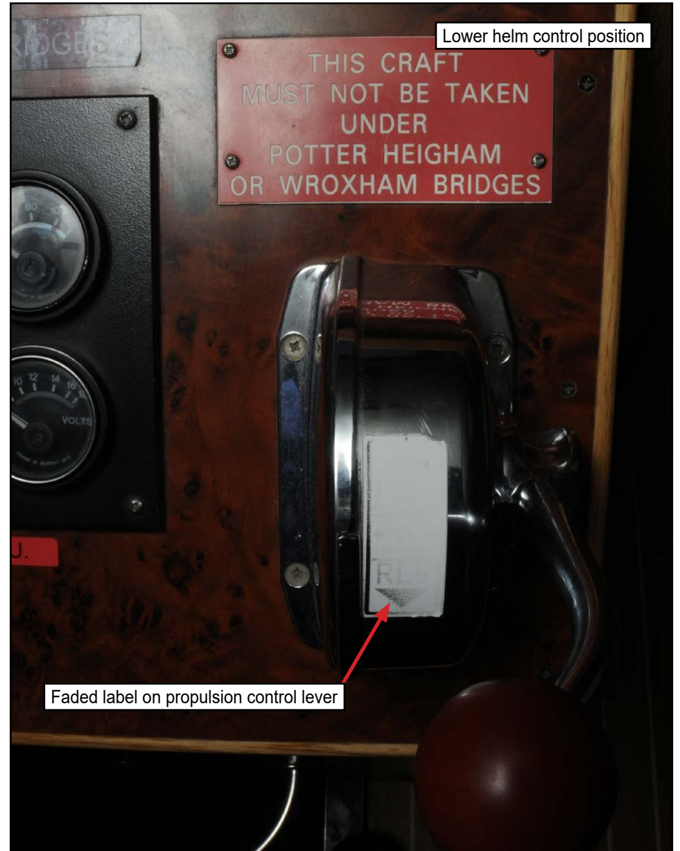
Figure 14: Faded propulsion control labelling at upper and lower helm control positions at time of Diamond Emblem 1 accident
