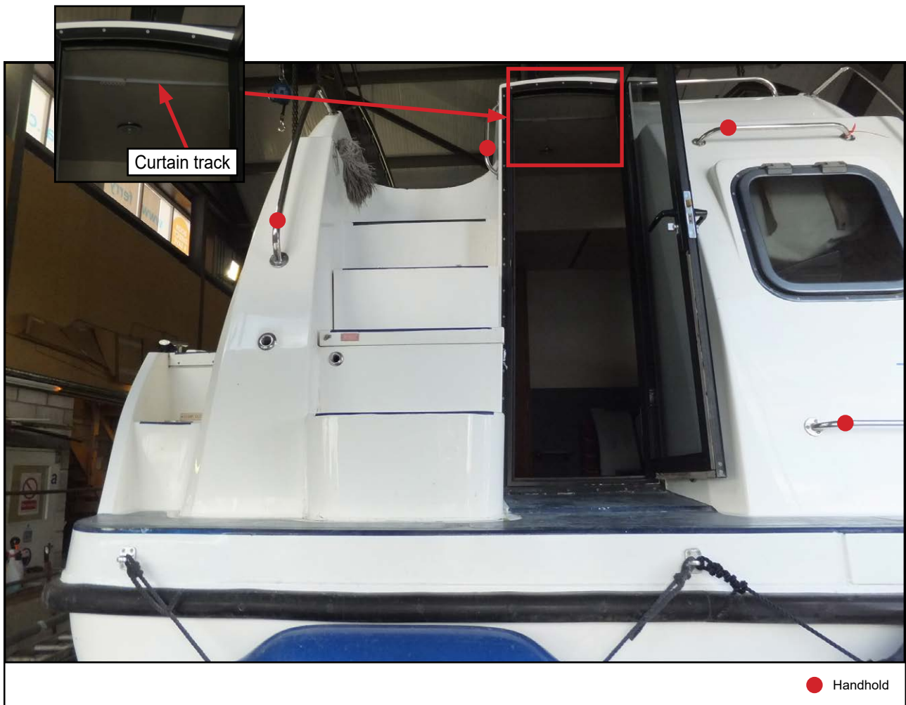
Figure 11: View of Diamond Emblem 1 stern, showing handholds and (inset) ceiling-mounted curtain track inside aft doorway
