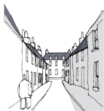
Limiting visual length by taller terminal building
