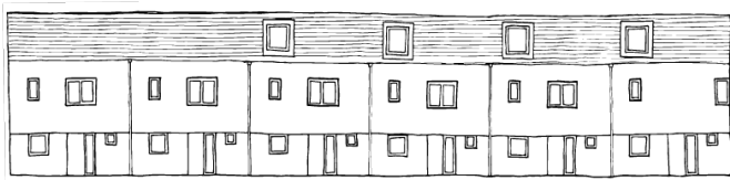
Front elevation with larger openings and facade subdivided to emphasise individual houses
