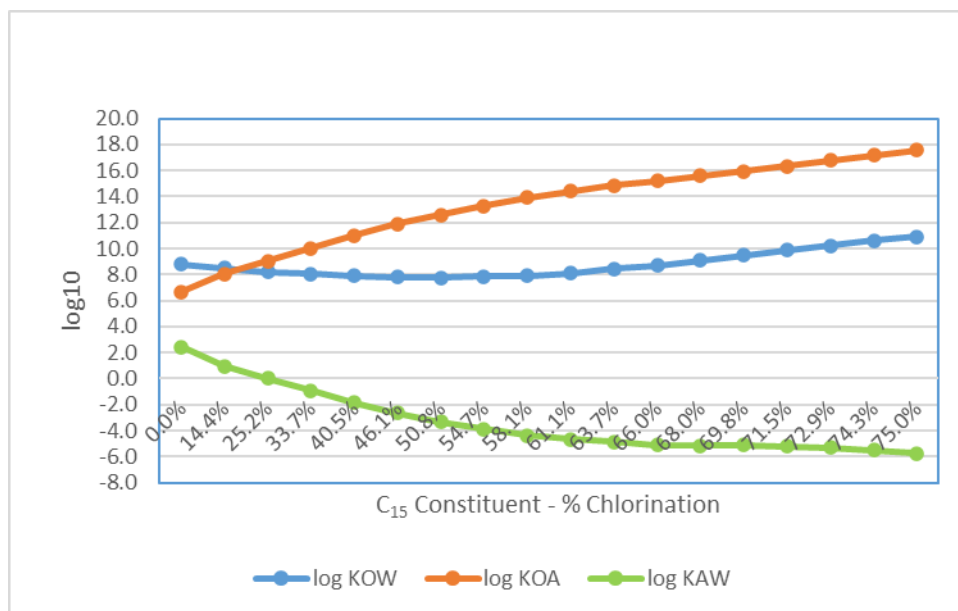
Figure 6: Plots of K OA , K OW and K AW for CPs - C 15 constituents (Endo, 2021)
