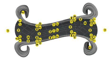
Figure 9 Model of the 3D printed bridge showing the location of sensors. Copyright: MX3D
