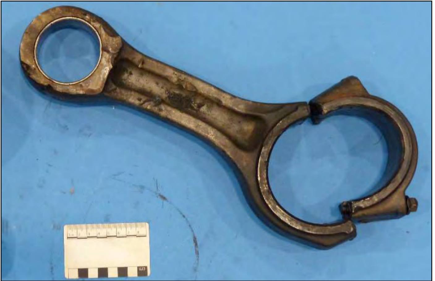
Figure 3: Failed connecting rod
