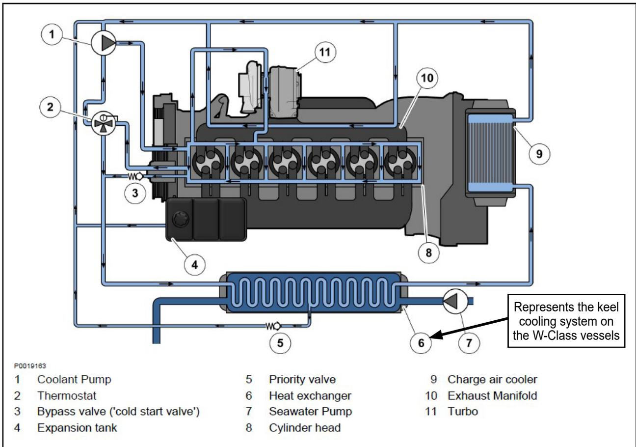
**Figure 14:** Engine cooling system
