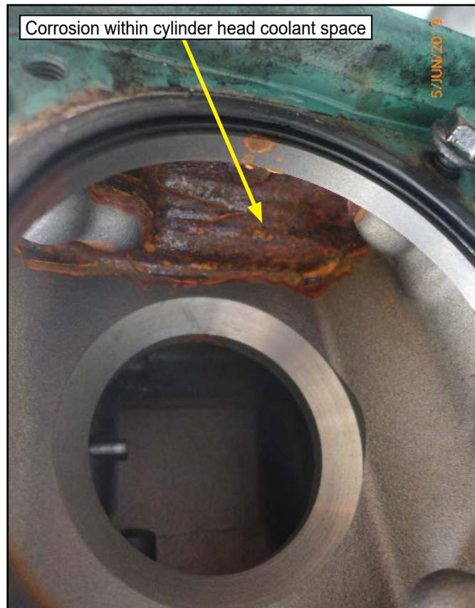
**Figure 32:** Corrosion in upper cylinder head from air pocket
