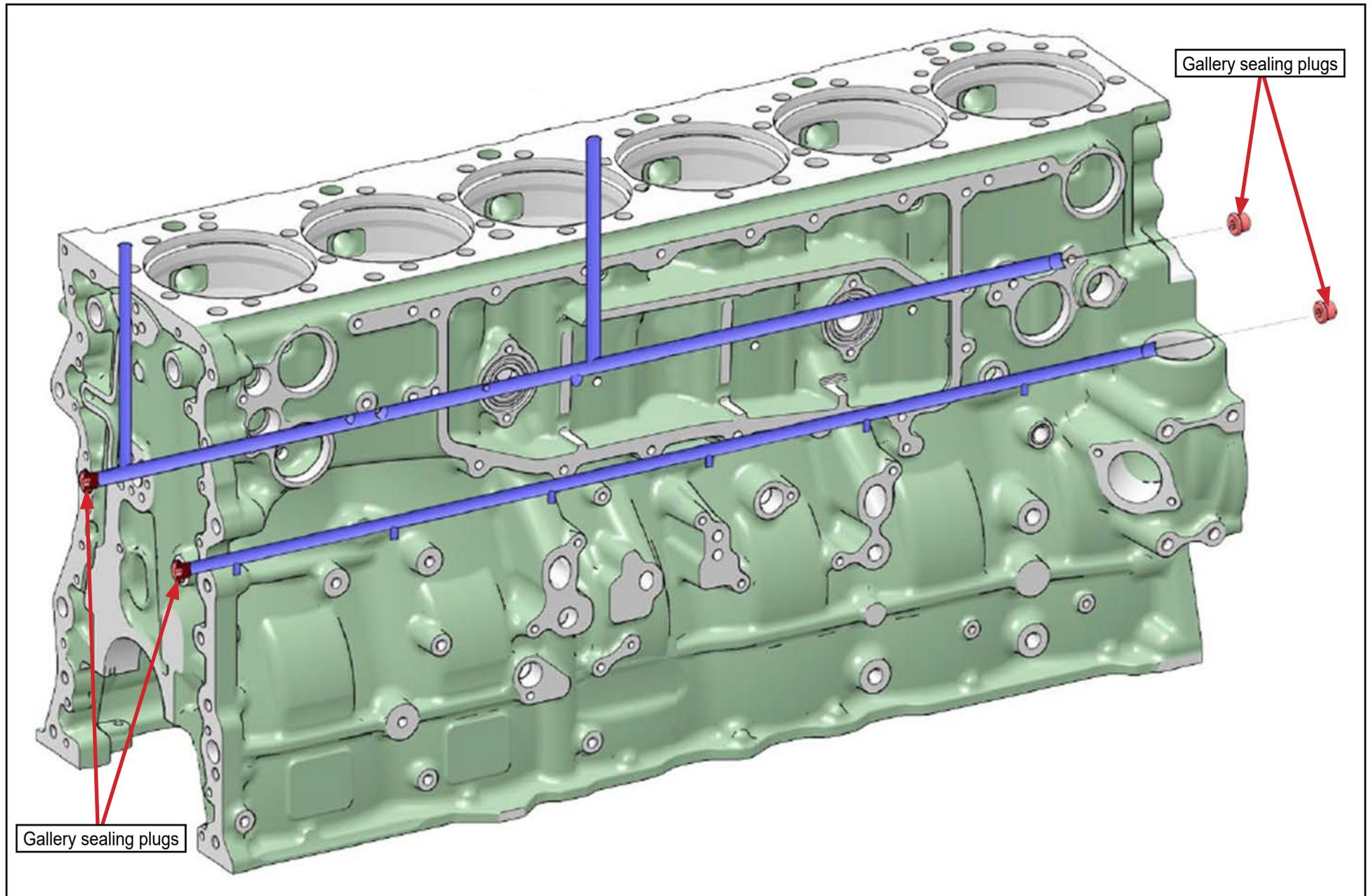
**Figure 18:** Engine block lubricating oil galleries
