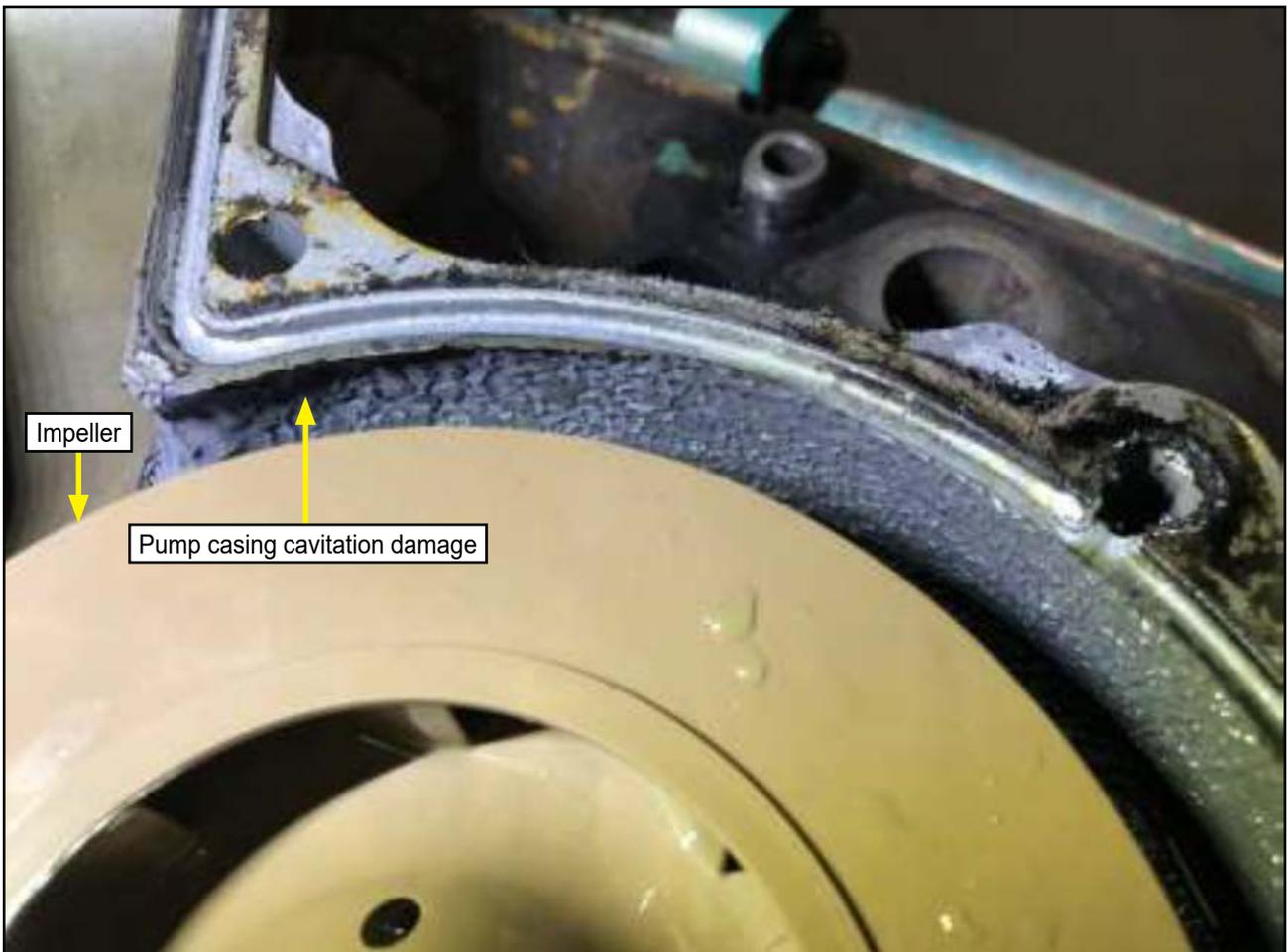
**Figure 31:** Cavitation erosion of high temperature cooling water pump
