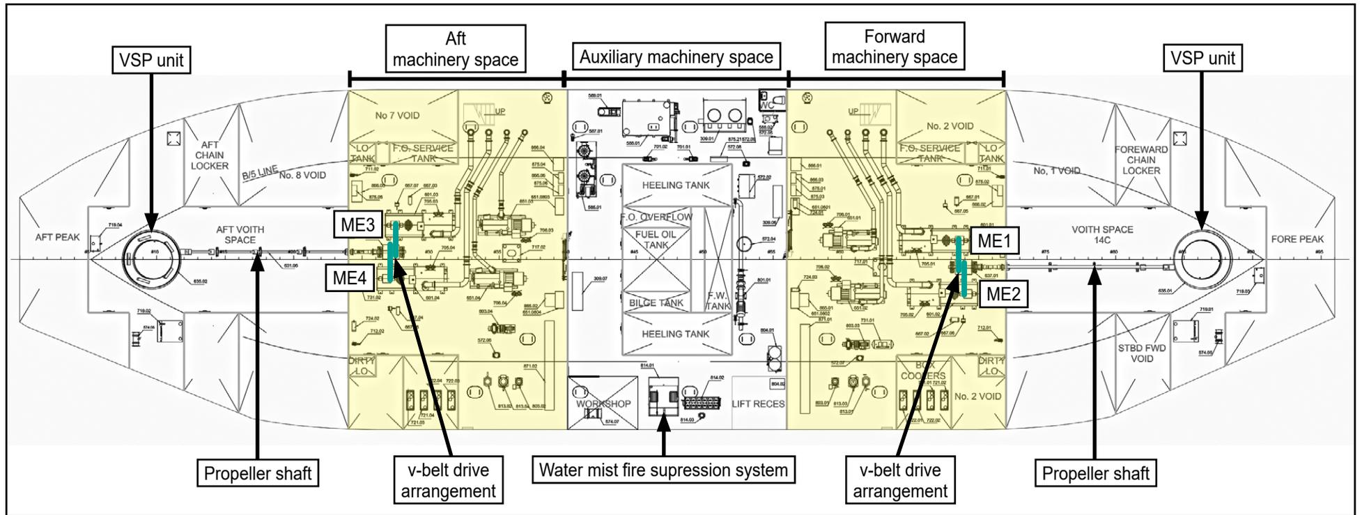
Figure 2: Layout of machinery spaces
