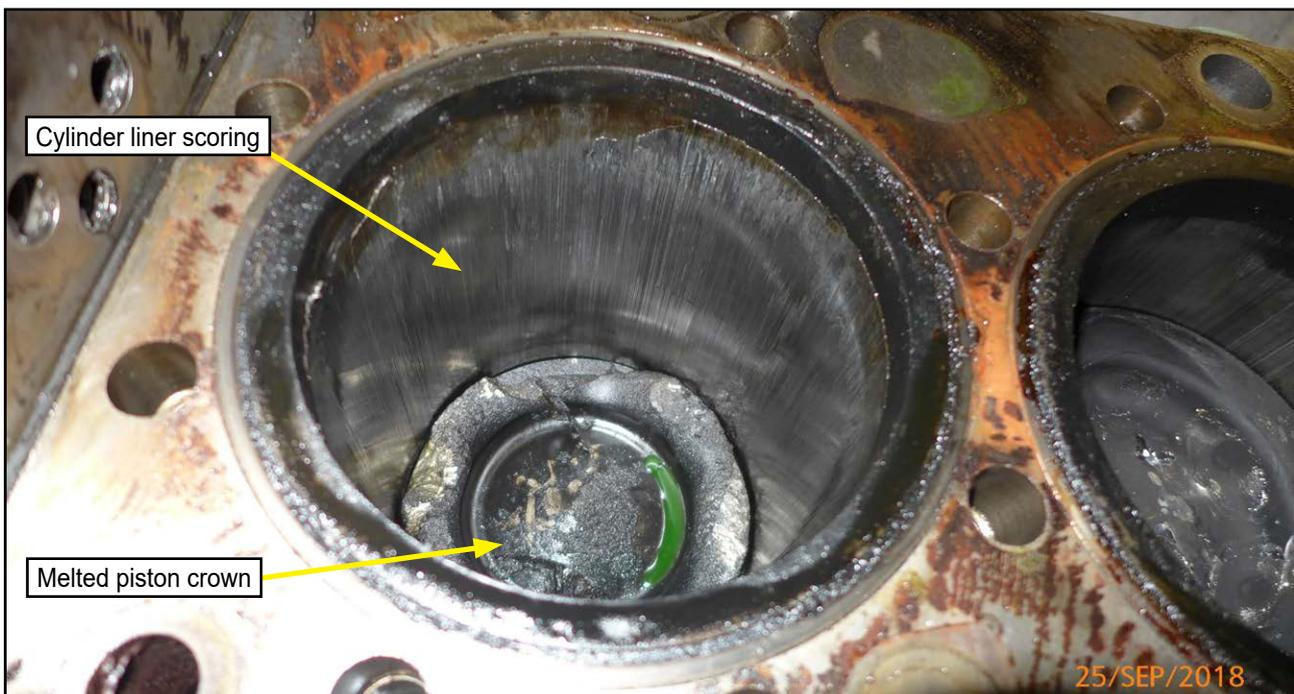
**Figure 23:** Event 3 – number six cylinder scoring and melted piston crown
