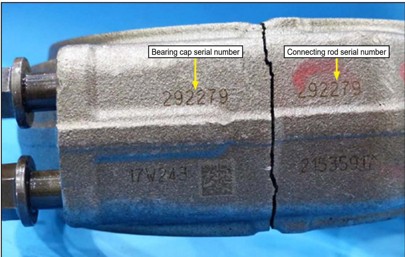
**Figure 8:** D16 MH bearing cap and connecting rod serial numbers
