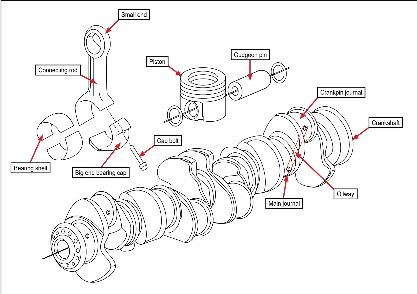
Figure 9: Schematic of rotating assembly
