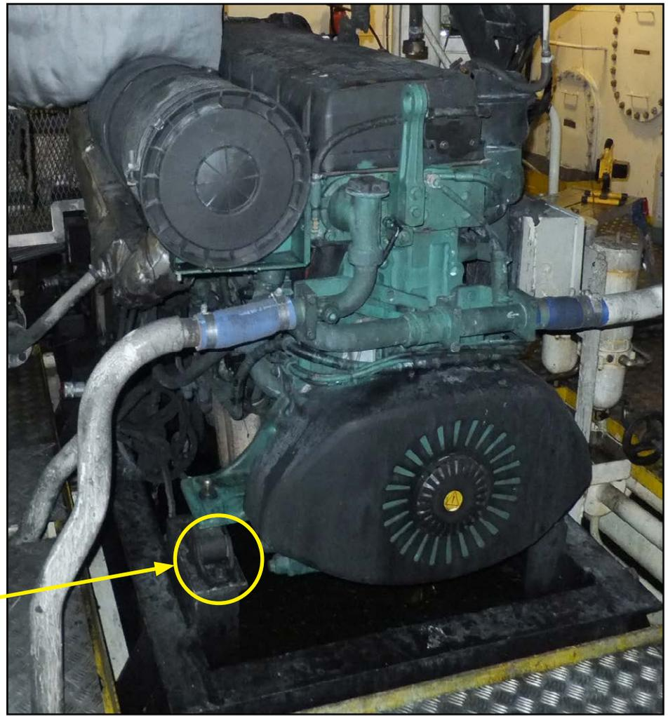
Figure 13: Flexible engine mounts
