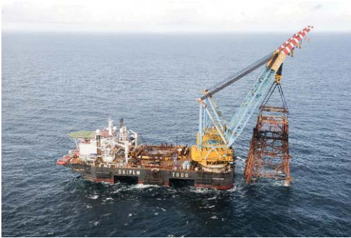
Figure 30. QP Jacket being transported to shore by S7000
