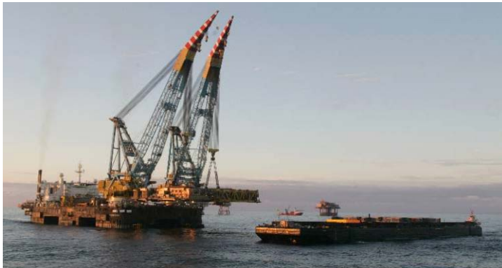
Figure 23. S7000 lifting TCP2 MSF in a single lift
