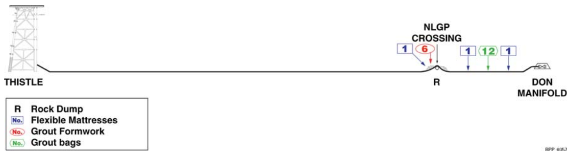
Figure 10.18 3in Chemical Injection Umbilical Stabilisation Features
