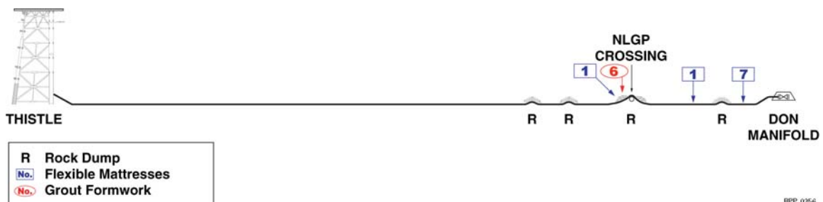
Figure 10.19 4in Control Umbilical Stabilisation Features
