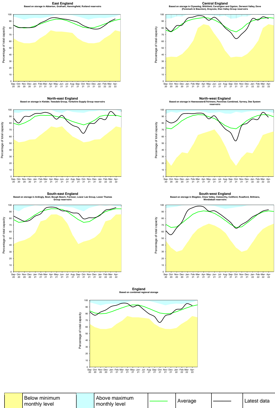
Figure 5.2: Regional reservoir stocks. End of month reservoir stocks compared to long term maximum, minimum and average stocks (Source: Water Companies). Note: Historic records of individual reservoirs/reservoir groups making up the regional values vary in length.
