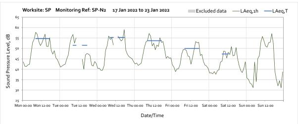
Note: Missing data throughout the week was due to battery falling below required voltage limit caused by prolonged insufficient sunlight.
