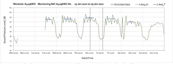
Note: Missing data between 06:00 on Monday 3<sup>rd</sup> January and 10:00 on Tuesday 4<sup>th</sup> January was due to battery falling below required voltage limit caused by prolonged insufficient sunlight.
