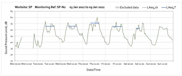
Note: Missing data between 08:00 and 18:00 on Monday 3<sup>rd</sup> January was due to battery falling below required voltage limit caused by prolonged insufficient sunlight.
