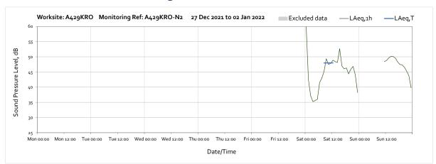
Note: High noise levels measured at 00:00 on Saturday 1st January were due to New Year Night celebration. Note: Missing data between 00:00 and 10:00 on Sunday 2nd January was due to battery falling below required voltage limit caused by prolonged insufficient sunlight.
