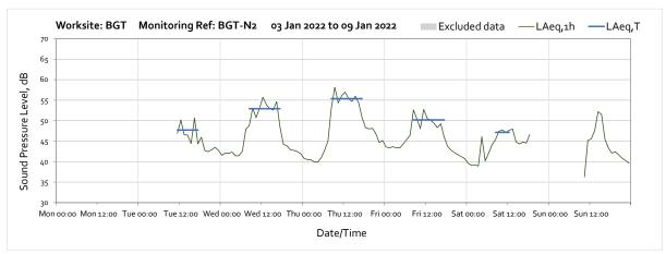
Note: Missing data throughout the week was due to battery falling below required voltage limit caused by prolonged insufficient sunlight.
