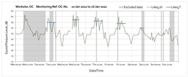
Note: Missing data at 09:00 on Wednesday 12<sup>th</sup> January was due to battery falling below required voltage limit caused by prolonged insufficient sunlight.
