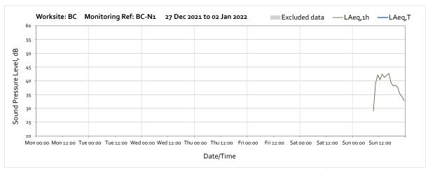
Note: Missing data between 00:00 on Saturday 1<sup>st</sup> January and 08:00 on Sunday 2<sup>nd</sup> January was due to battery falling below required voltage limit caused by prolonged insufficient sunlight.
