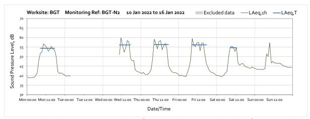
Note: Missing data between 04:00 on Tuesday 11<sup>th</sup> January and 09:00 on Wednesday 12<sup>th</sup> January was due to battery falling below required voltage limit caused by prolonged insufficient sunlight.
