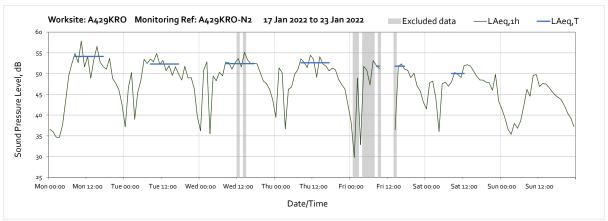
Note: Missing data between 10:00 and 13:00 on Friday 21st January was due to battery falling below required voltage limit caused by prolonged insufficient sunlight.
