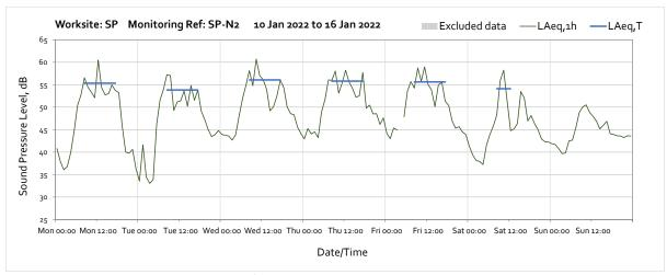
Note: Missing data at 04:00 on Friday 14<sup>th</sup> January was due to battery falling below required voltage limit caused by prolonged insufficient sunlight.
