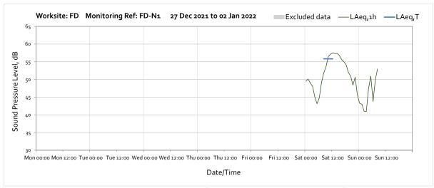
Note: Missing data in between 09:00 on Sunday 2<sup>nd</sup> January and 10:00 on Tuesday 11<sup>th</sup> January was due to battery falling below required voltage limit caused by prolonged insufficient sunlight.
