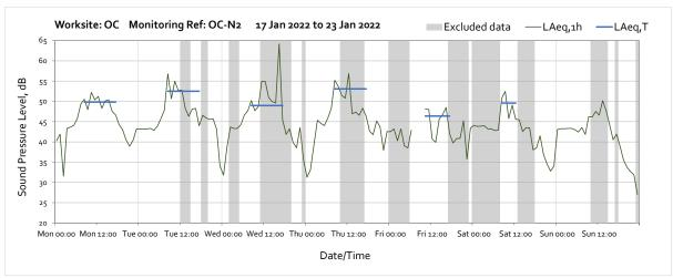
Note: Missing data between 07:00 and 09:00 on Friday 21st January was due to battery falling below required voltage limit caused by prolonged insufficient sunlight.
