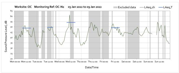
Note: Missing data throughout the week was due to battery falling below required voltage limit caused by prolonged insufficient sunlight.
