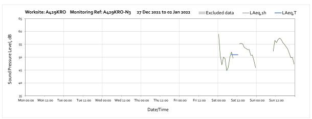
Note: High noise levels measured at 00:00 on Saturday 1st January were due to New Year Night celebration. Note: Missing data throughout the week was due to battery falling below required voltage limit caused by prolonged insufficient sunlight.
