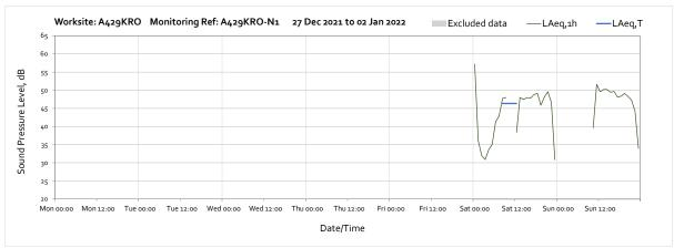
Note: High noise levels measured at 00:00 on Saturday 1st January were due to New Year Night celebration. Note: Missing data throughout the week was due to battery falling below required voltage limit caused by prolonged insufficient sunlight.
