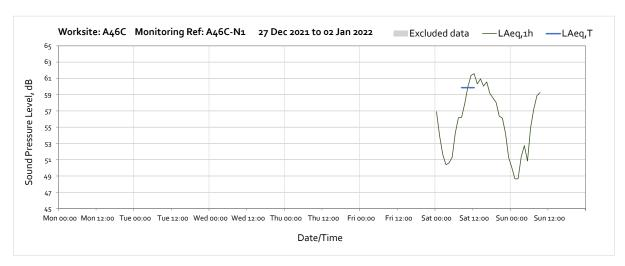
Note: Missing data from 09:00 on 2<sup>nd</sup> January to the end of the month due to on-going issues with the meter and access restrictions to the monitoring station to address the issue.
