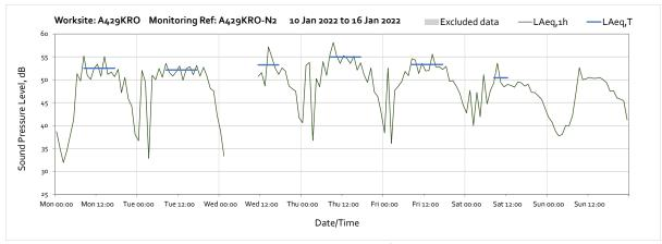
Note: Missing data between 02:00 and 10:00 on Wednesday 12<sup>th</sup> January was due to battery falling below required voltage limit caused by prolonged insufficient sunlight.
