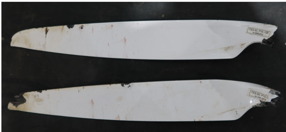
Figure 9 Propeller blade damage
