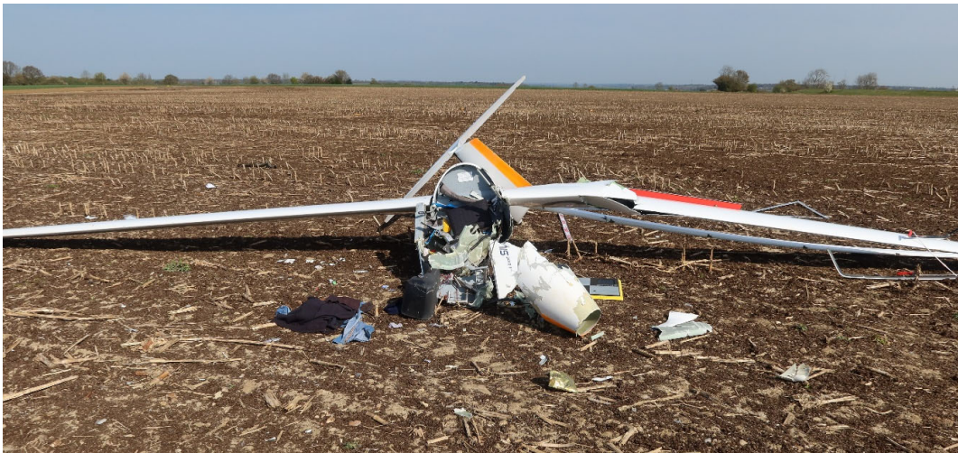
Figure 2 Damage to the aircraft
