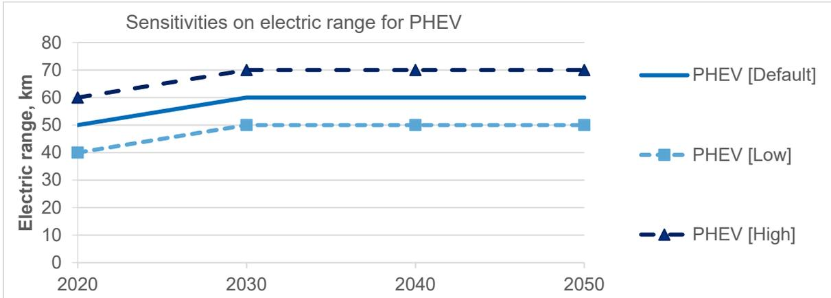
**Figure A9: WLTP light duty vehicle utility function (UF), used to estimate share of operation in electric mode given the vehicle electric range, plus high/low sensitivities used in the analysis**
