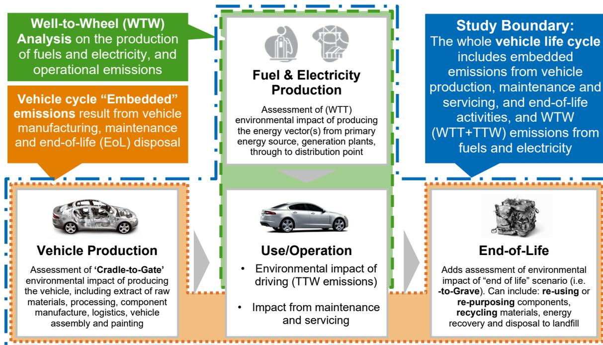
Note: Infrastructure for energy production (electricity and fuels) is also included. Electricity storage is excluded. WTT = Well-to-Tank; TTW = Tank-to-Wheel.
