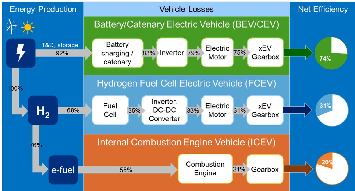
Notes: Illustrative schematic view based on typical conversion efficiencies, produced by Ricardo. e-fuels are produced by 'power-to-liquids' (PtL) process using hydrogen produced from electrolysis of water, captured CO<sub>2</sub> (from the air or other sources) and Fischer-Tropsch synthesis.
