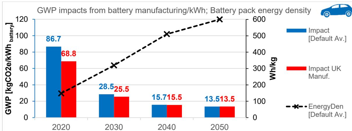
Figure A25: Sensitivity on battery and vehicle production, Lower Medium Car, Net Zero Power Scenario – BEV manufacturing (total) GWP impacts [in kgCO<sub>2</sub>e/vkm (lifetime)] and battery energy density [in Wh/kg]
