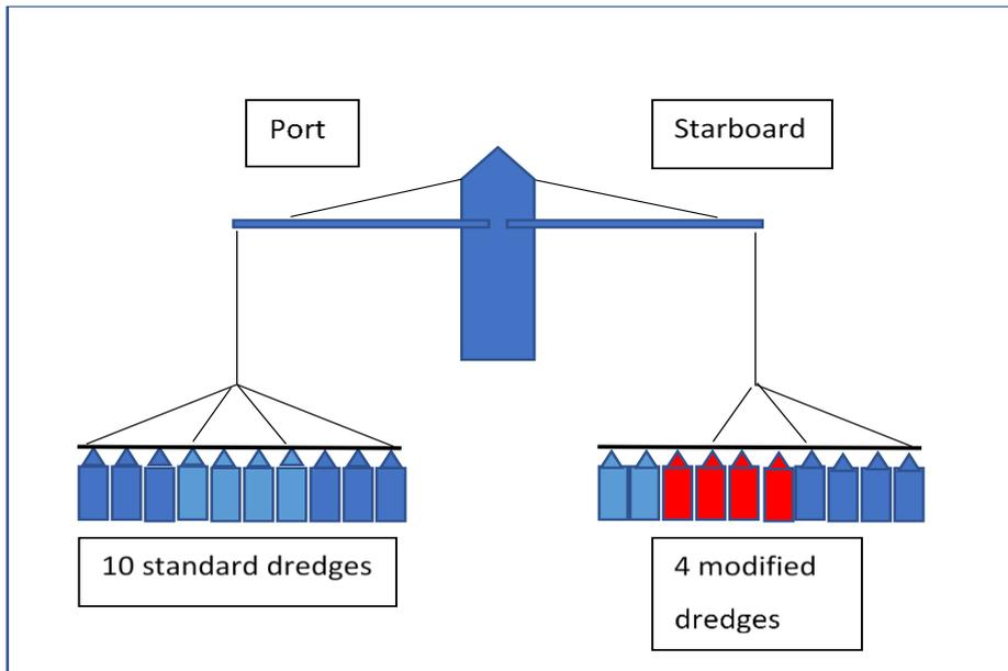
Figure 1.3: Gear configuration on the survey vessel.
