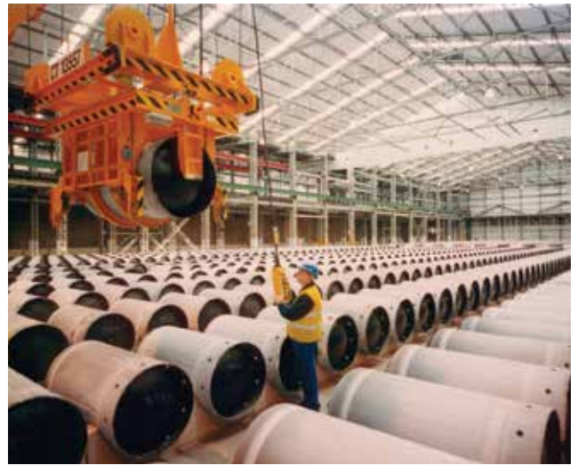
Hexafluoride drums being stored at Capenhurst
