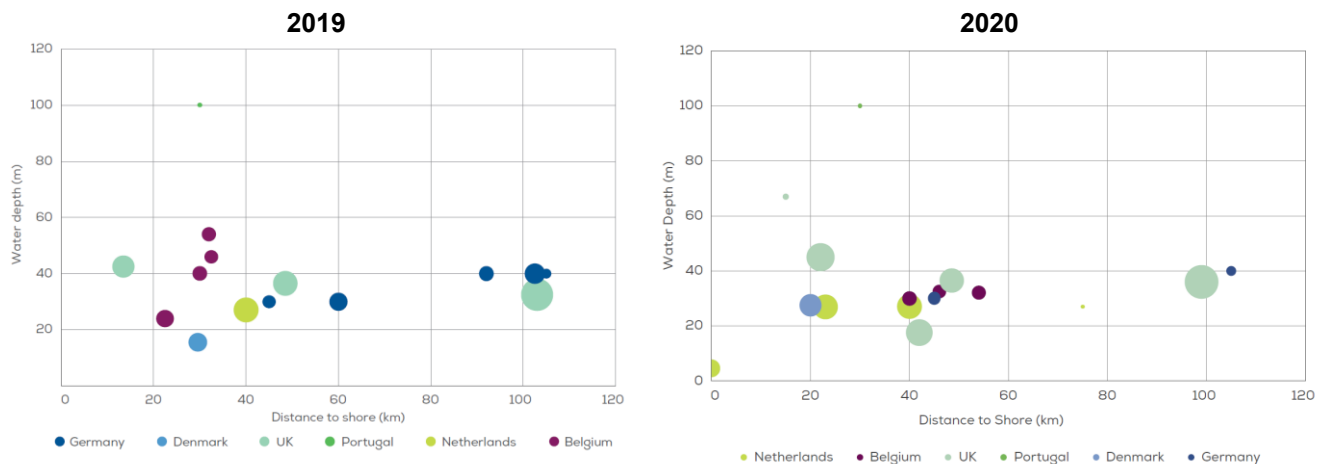
Figure 5.52: Average water depth and distance to shore of offshore wind farms under construction
