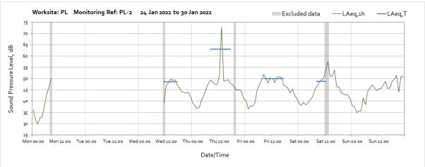
Note: Missing data between 09:00 on Monday 24<sup>th</sup> January and 11:00 on Wednesday 26<sup>th</sup> January were due to loss of power to the monitor caused by insufficient sunlight to charge ancillary batteries.
