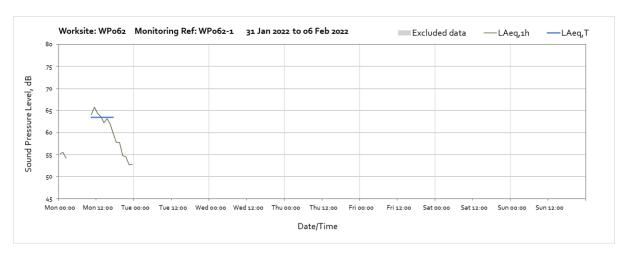
Note: Missing data between 03:00 and 10:00 on Monday 31st January were due to loss of power to the monitor caused by insufficient sunlight to charge ancillary batteries.
