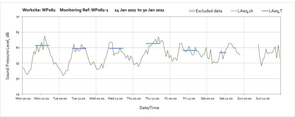
Note: Missing data between 22:00 on Saturday 29<sup>th</sup> January and 09:00 on Sunday 30<sup>th</sup> January were due to loss of power to the monitor caused by insufficient sunlight to charge ancillary batteries.
