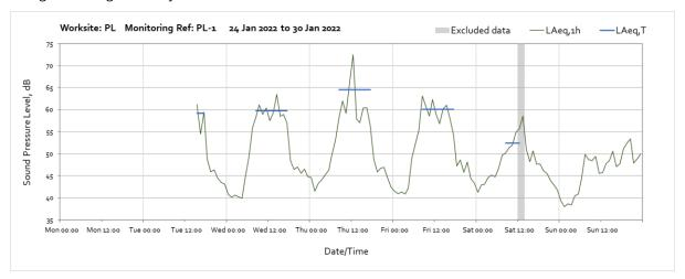
Note: Missing data between 09:00 on Sunday 9<sup>th</sup> January and 15:00 on Tuesday 25<sup>th</sup> January were due to loss of power to the monitor caused by insufficient sunlight to charge ancillary batteries.
