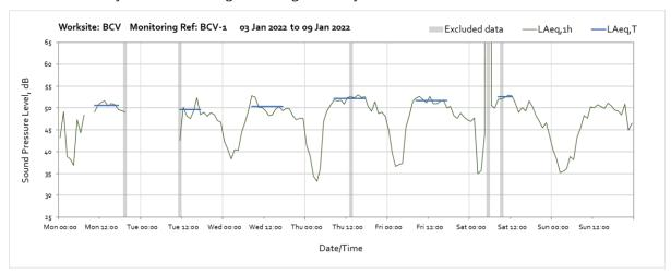
Note: Missing data throughout the week were due to loss of power to the monitor caused by insufficient sunlight to charge ancillary batteries. High noise levels between 05:00 and 06:00 on Saturday 9<sup>th</sup> January was due to failure of connection between meter and server.
