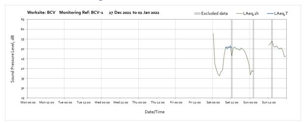
Note: Missing data between 03:00 and 12:00 on Sunday 2<sup>nd</sup> January were due to loss of power to the monitor caused by insufficient sunlight to charge ancillary batteries.
