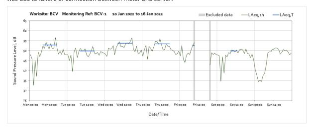
Note: Missing data between 10:00 and 19:00 on Friday  $14^{th}$  January were due to loss of power to the monitor caused by insufficient sunlight to charge ancillary batteries.
