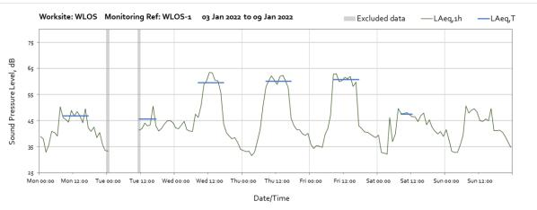
Note: Missing data between 01:00 and 11:00 on Tuesday 4<sup>th</sup> January were due to loss of power to the monitor caused by insufficient sunlight to charge ancillary batteries.
