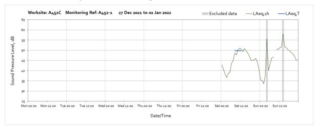
Note: Missing data between 09:00 and 10:00 on Sunday 2<sup>nd</sup> January were due to loss of power to the monitor caused by insufficient sunlight to charge ancillary batteries.
