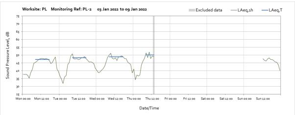
Note: Missing data between 14:00 on Thursday 6<sup>th</sup> January and 12:00 on Sunday 9<sup>th</sup> January were due to loss of power to the monitor caused by insufficient sunlight to charge ancillary batteries.
