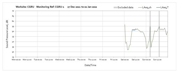
Note: Missing data throughout the week were due to loss of power to the monitor caused by insufficient solar energy to charge ancillary batteries.
