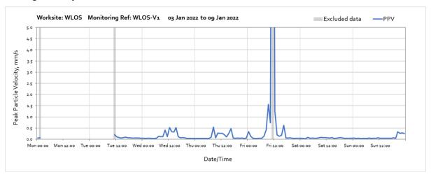
Note: Missing data during the week were due to loss of power to the monitor caused by insufficient sunlight to charge ancillary batteries. High vibration measured on 11:00 Friday 7<sup>th</sup> January was due to local disturbace and is not related to HS2 works.
