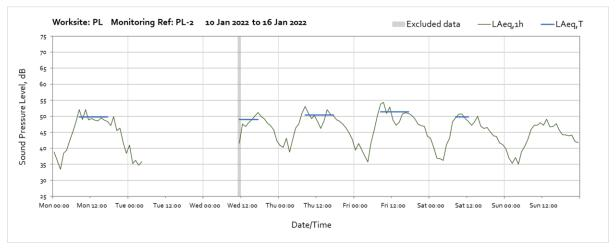
Note: Missing data between 05:00 on Tuesday 11<sup>th</sup> January and 11:00 on Wednesday 12<sup>th</sup> January were due to loss of power to the monitor caused by insufficient sunlight to charge ancillary batteries.
