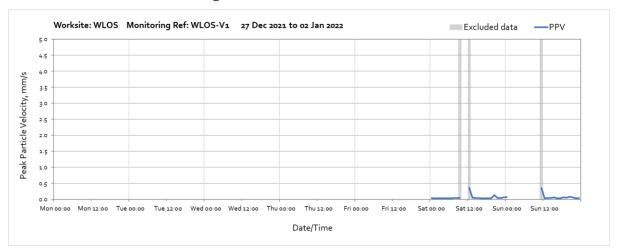
Note: Missing data during the week were due to loss of power to the monitor caused by insufficient sunlight to charge ancillary batteries.
