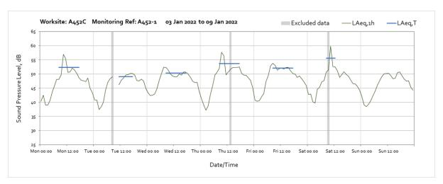
Note: Missing data between 09:00 and 11:00 on Tuesday  $4^{th}$  January were due to loss of power to the monitor caused by insufficient sunlight to charge ancillary batteries.
