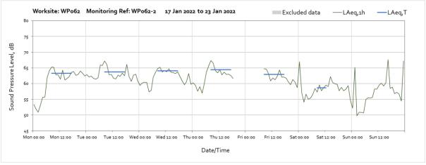
Note: Missing data between 19:00 on Thursday 20<sup>th</sup> January and 08:00 on Friday 21<sup>st</sup> January were due to loss of power to the monitor caused by insufficient sunlight to charge ancillary batteries.
