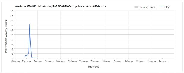
Note: Higher vibration levels measured during the week were due to plant movements and piling works. Missing data between 16:00 on Saturday 29<sup>th</sup> and 09:00 on Monday 31<sup>st</sup> January 2022 was due to battery falling below required voltage limit caused by prolonged insufficient sunlight.
