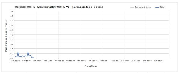
Note: Missing data from 21:00 on Monday 31<sup>st</sup> January 2022 onwards was due to a fence falling on the cable of the monitor.
