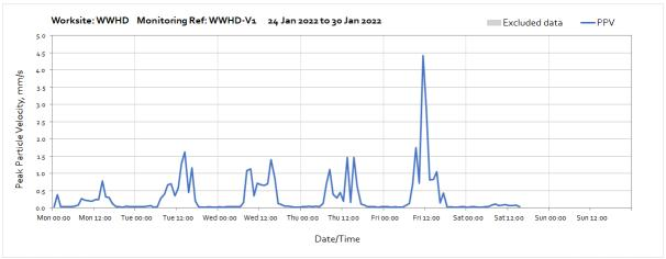
Note: High vibration levels measured during the week were due to plant movements and piling works. Missing data between 16:00 on Saturday 29<sup>th</sup> and 09:00 on Monday 31<sup>st</sup> January 2022 was due to battery falling below required voltage limit caused by prolonged insufficient sunlight.
