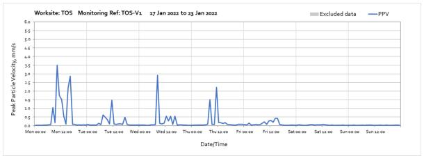
Note: Higher vibration levels measured across the week were due to asphalting works of the site haul road undertaken close to the monitoring location. The nearest receptor is further away and therefore vibration levels will be lower at the receptor location.
