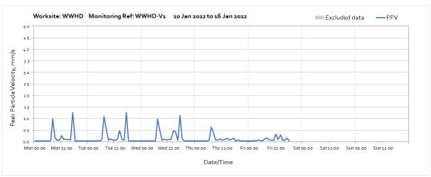
Note: Missing data between 19:00 on Friday 14<sup>th</sup> and 11:00 on Monday 17<sup>th</sup> January 2022 was due to battery falling below required voltage limit caused by prolonged insufficient sunlight.
