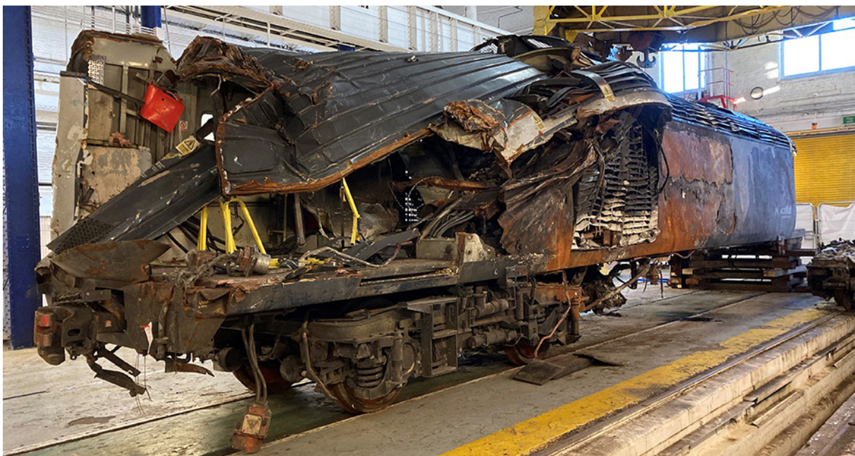
Figure 87: Fire-damaged leading power car
