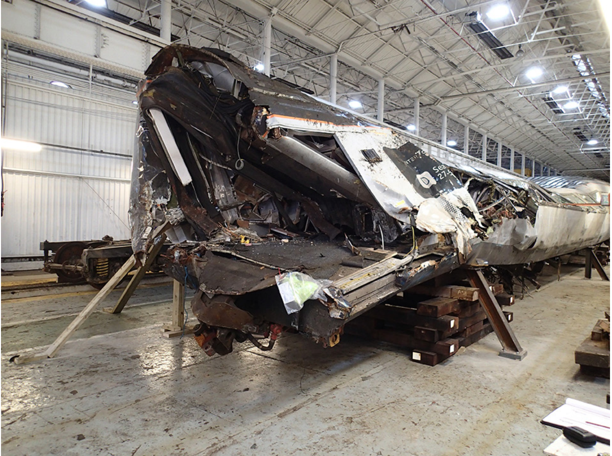
Figure 74: Damage to leading end of coach D
