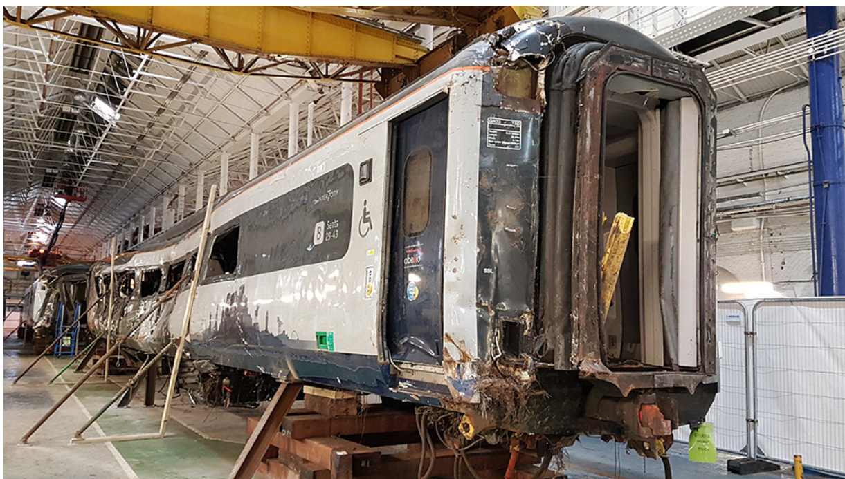
Figure 78: Damage to leading end and right side of coach B
