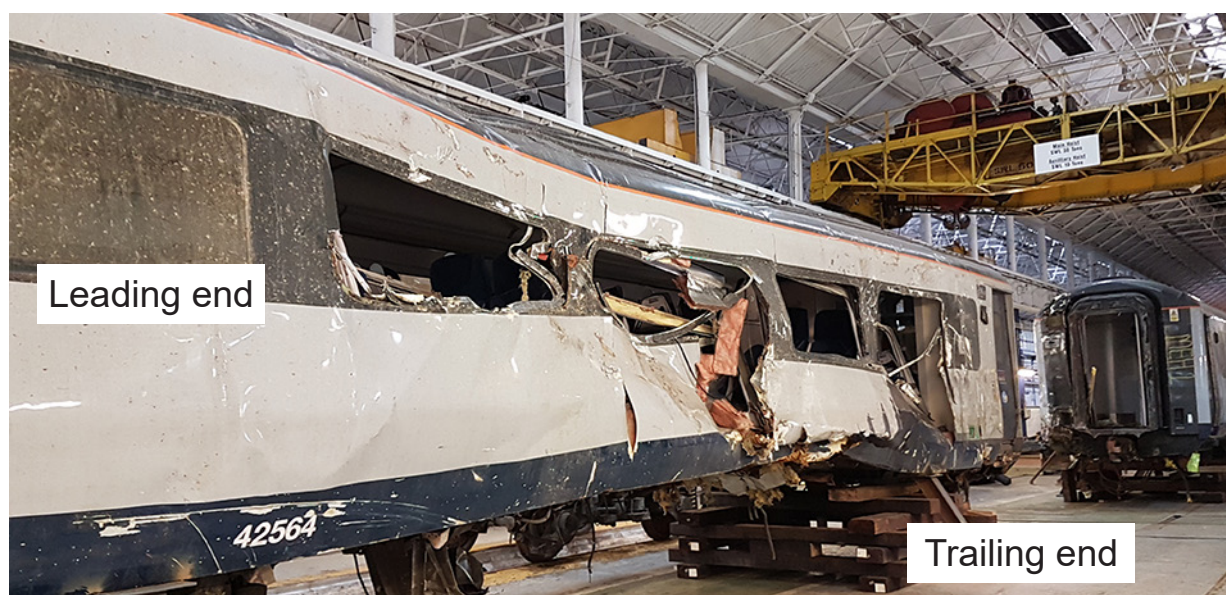
Figure 77: Penetration damage at trailing end of coach C (left side)
