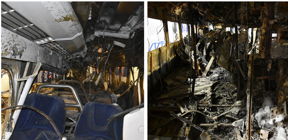
Fire damage in the third coach
