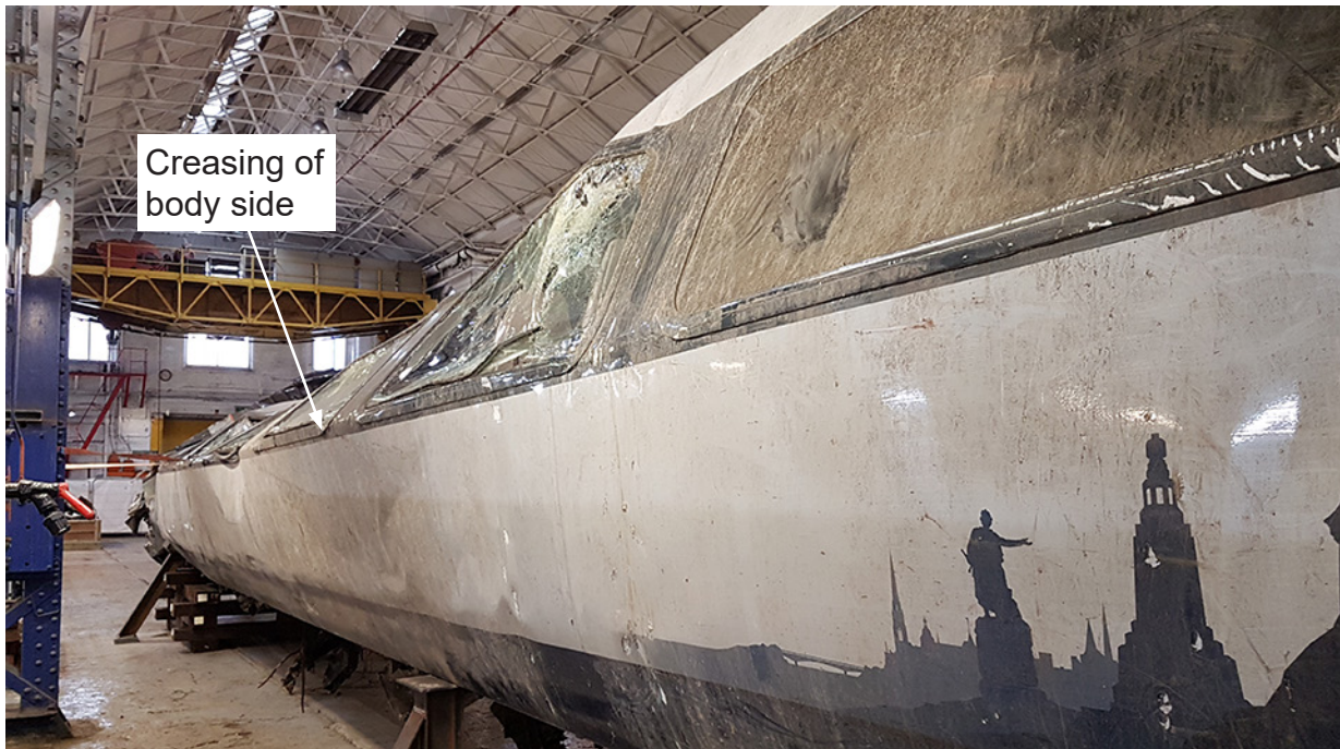
Figure 81: Creasing along left-hand bodyside of coach D
