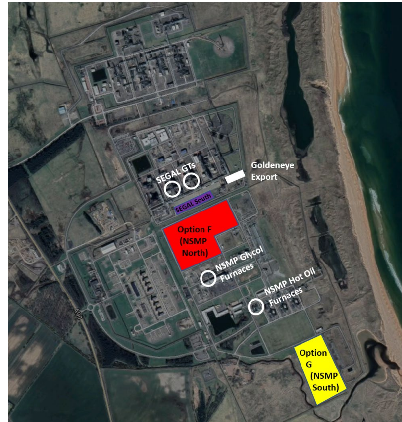
Figure 1-1: Options shortlist; Options I and J (not shown) are combinations of Compression at NSMP South and capture at SEGAL South and NSMP North respectively
