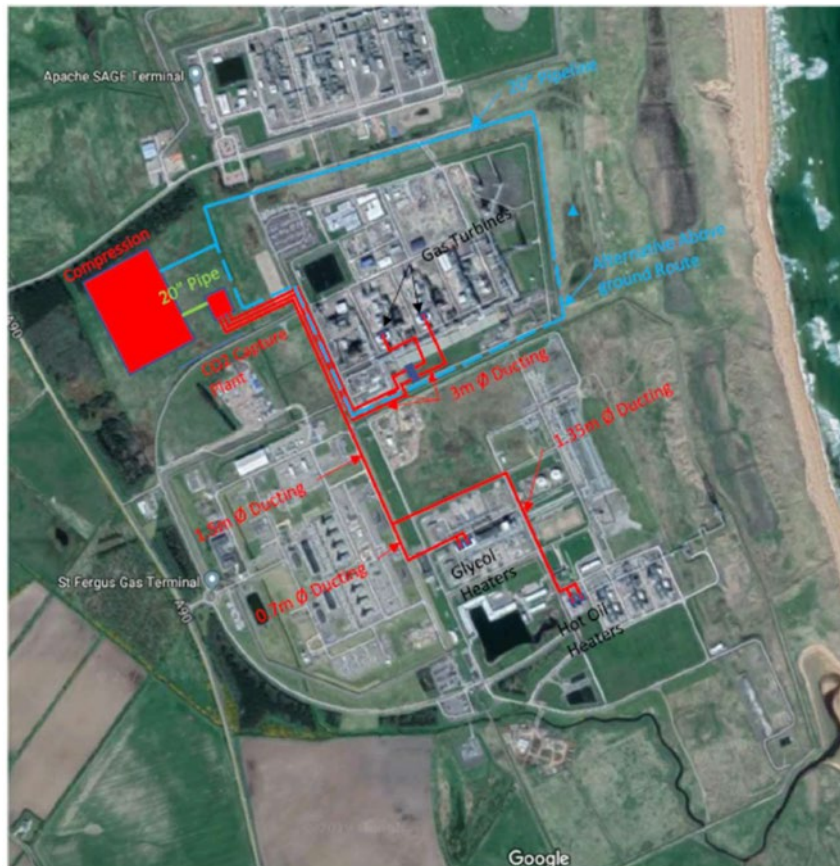
Figure 5-5: Preliminary Ductwork and Pipeline Routing for Blackhill
