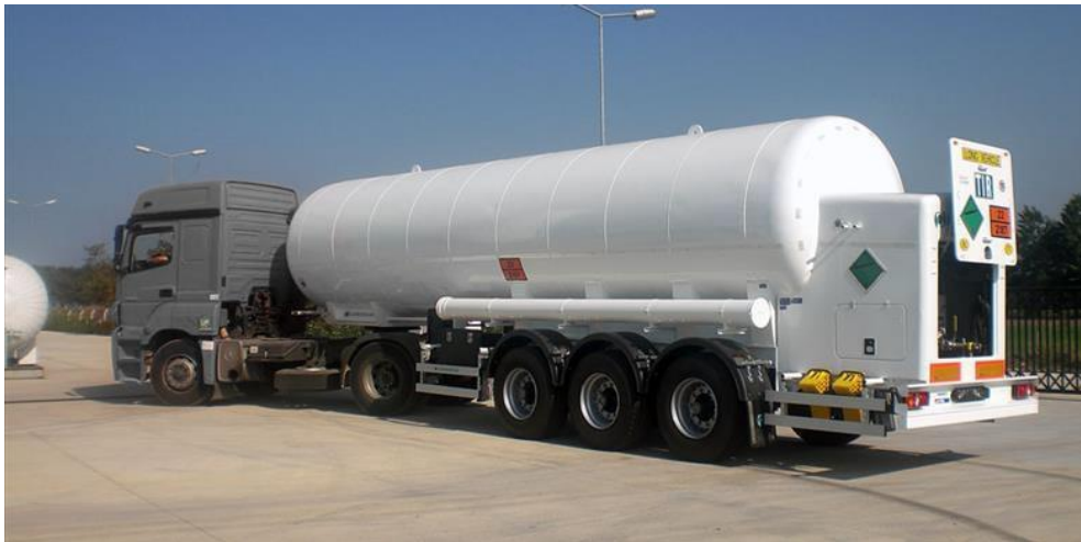
Figure 2-7 – CO 2 road tanker trailer manufactured by Karbonsan
