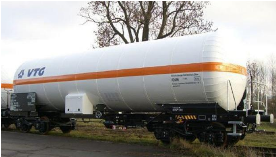
Figure 2-8 - CO 2 railcar, operated by VTG AG
