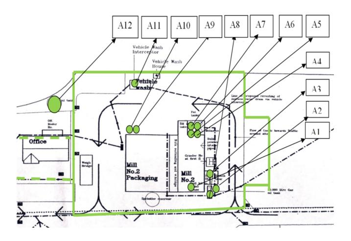
Installation Boundary Wastewater Drainage Route Emissions to air
