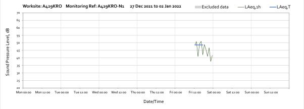
Note: Missing data between 00:00 on Monday 20<sup>th</sup> December and 11:00 on Friday 31<sup>st</sup> of December was due to prolonged insufficient solar power to the equipment. To ensure there is no loss of power again solar maintenance is being conducted.
