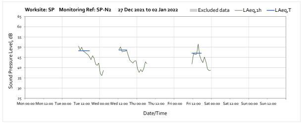
Note: Missing data throughout the week were due to prolonged insufficient solar power to the equipment. To ensure there is no loss of power again solar maintenance is being conducted.
