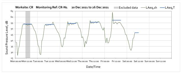
Note: Missing data in between 09:00 on Saturday 25<sup>th</sup> December and 09:00 on Friday 31<sup>st</sup> December were due to prolonged insufficient solar power to the equipment. To ensure there is no loss of power again solar maintenance is being conducted.
