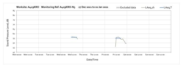
Note: Missing data in between 19:00 on Wednesday 29<sup>th</sup> December and 10:00 on on Friday 31<sup>st</sup> December were due to prolonged insufficient solar power to the equipment. To ensure there is no loss of power again solar maintenance is being conducted.
