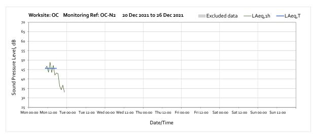
Note: Missing data in between 23:00 on Monday 20<sup>th</sup> December and 09:00 on Friday 31<sup>st</sup> December were due to prolonged insufficient solar power to the equipment. To ensure there is no loss of power again solar maintenance is being conducted.
