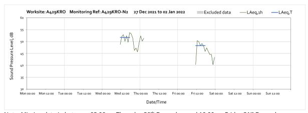
Note: Missing data in between 03:00 on Thursday 30<sup>th</sup> December and 10:00 on Friday 31<sup>st</sup> December were due to prolonged insufficient solar power to the equipment. To ensure there is no loss of power again solar maintenance is being conducted.
