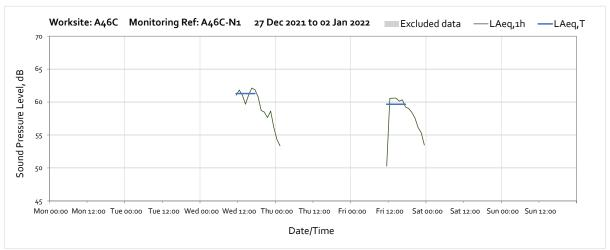
Note: Missing data throughout the week until 10:00 on Wednesday 29<sup>th</sup> December were due to prolonged insufficient solar power to the equipment. To ensure there is no loss of power again solar maintenance is being conducted.
