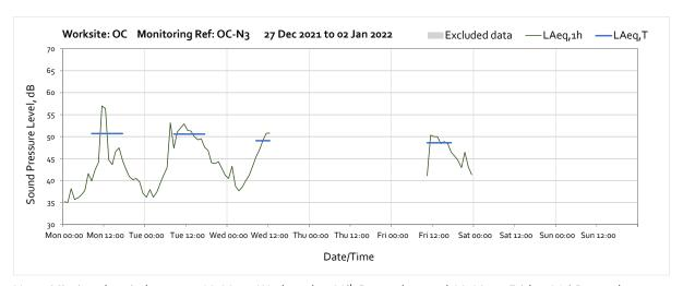
Note: Missing data in between 13:00 on Wednesday 29<sup>th</sup> December and 09:00 on Friday 31<sup>st</sup> December were due to prolonged insufficient solar power to the equipment. To ensure there is no loss of power again solar maintenance is being conducted.
