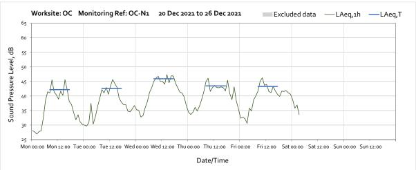
Note: Missing data in between 04:00 on Saturday 25<sup>th</sup> December and 09:00 on Friday 31<sup>st</sup> December were due to prolonged insufficient solar power to the equipment. To ensure there is no loss of power again solar maintenance is being conducted.
