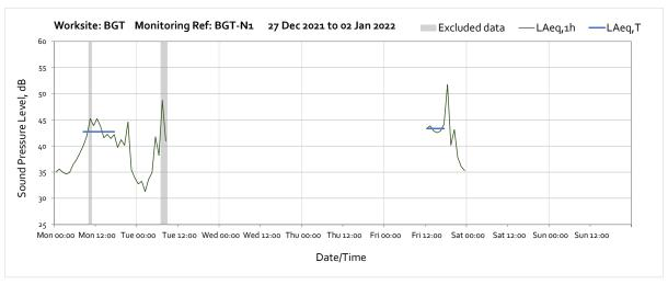
Note: Missing data between 09:00 on Tuesday 28<sup>th</sup> December and 11:00 on Friday 31<sup>st</sup> of December was due to prolonged insufficient solar power to the equipment. To ensure there is no loss of power again solar maintenance is being conducted.
