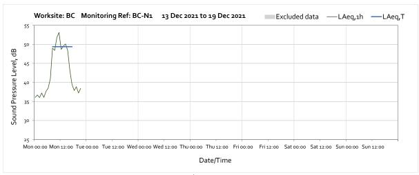
Note: Missing data between 22:00 on Monday 13<sup>th</sup> December and 23:00 on Friday 31<sup>st</sup> of December was due to prolonged insufficient solar power to the equipment. To ensure there is no loss of power again solar maintenance is being conducted.
