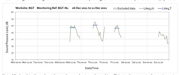
Note: Missing data throughout the week were due to prolonged insufficient solar power to the equipment.
