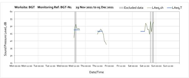
Note: Missing data throughout the week were due to prolonged insufficient solar power to the equipment.
