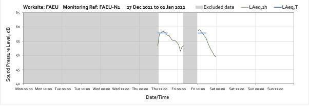
Note: Missing data in between 04:00 and 11:00 on Friday 31st December was due to battery falling below the required voltage limit caused by prelonged insufficient sunlight.
