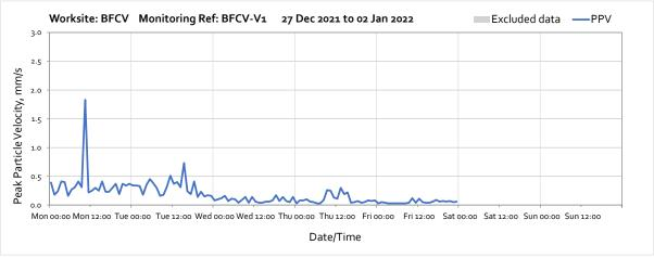
Note: High vibration levels measured at 10:00 on Monday 27<sup>th</sup> December were due to construction works undertaken near the monitoring station.
