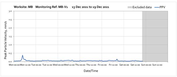
Note: Missing data in between 21:00 on Saturday 18<sup>th</sup> December and15:00 on Tuesday 21<sup>st</sup> December was due to battery falling below the required voltage limit caused by prelonged insufficient sunlight. Batteries were replaced on 23<sup>rd</sup> December 2021.
