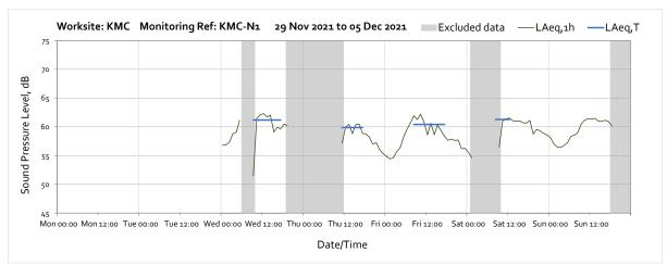
Note: Missing data throughout the week was due to battery falling below the required voltage limit caused by prelonged insufficient sunlight. Batteries were replaced on 9<sup>th</sup> December 2021.
