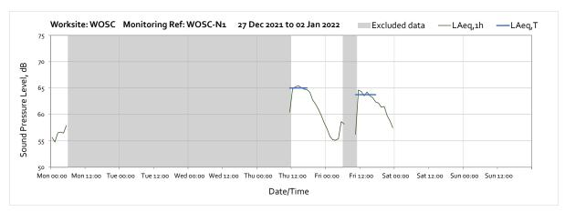
Note: Missing data throughout the week was due to battery falling below the required voltage limit caused by prolonged insufficient sunlight.
