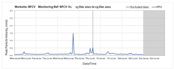
Note: High vibration levels measured at 17:00 on Wednesday 15<sup>th</sup> December were due to construction works undertaken near the monitoring station.
