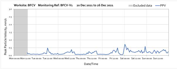
Note: Missing data in between 00:00 on Sunday 19<sup>th</sup> December and13:00 on Monday 20<sup>th</sup> December was due to battery falling below the required voltage limit caused by prelonged insufficient sunlight.
