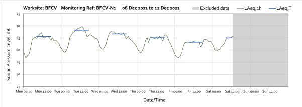
Note: Missing data in between 14:00 on Saturday 11<sup>th</sup> December and 16:00 on Wednesday 15<sup>th</sup> December was due to battery falling below the required voltage limit caused by prelonged insufficient sunlight.
