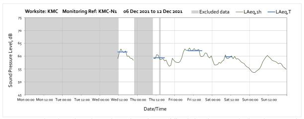
Note: Missing data throughout the week was due to battery falling below the required voltage limit caused by prelonged insufficient sunlight. Batteries were replaced on 9<sup>th</sup> December 2021.
