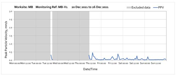
Note: Missing data in between 19:00 on Tuesday 21<sup>st</sup> December and 09:00 on Thursday 23<sup>rd</sup> December was due to battery falling below the required voltage limit caused by prelonged insufficient sunlight. Batteries were replaced on 23<sup>rd</sup> December 2021.
