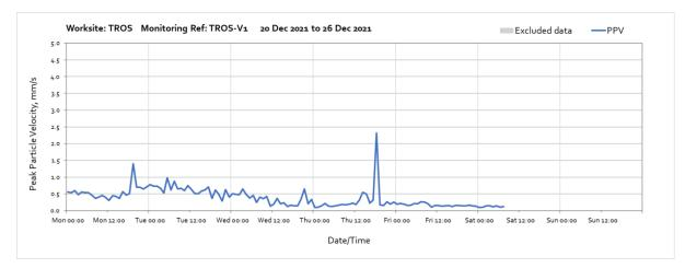
Note: Equipment power problems arising from weak sunlight caused the above missing data.
