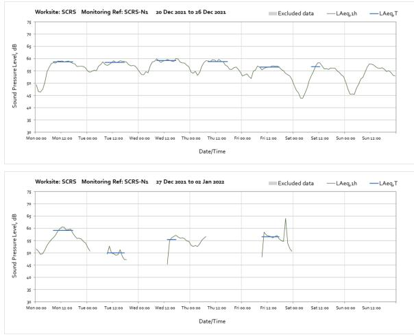
Note: Equipment power problems arising from weak sunlight caused the above missing data.
