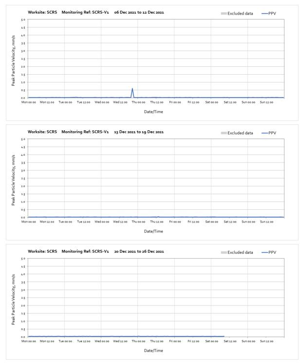
Note: Equipment power problems arising from weak sunlight caused the above missing data.
