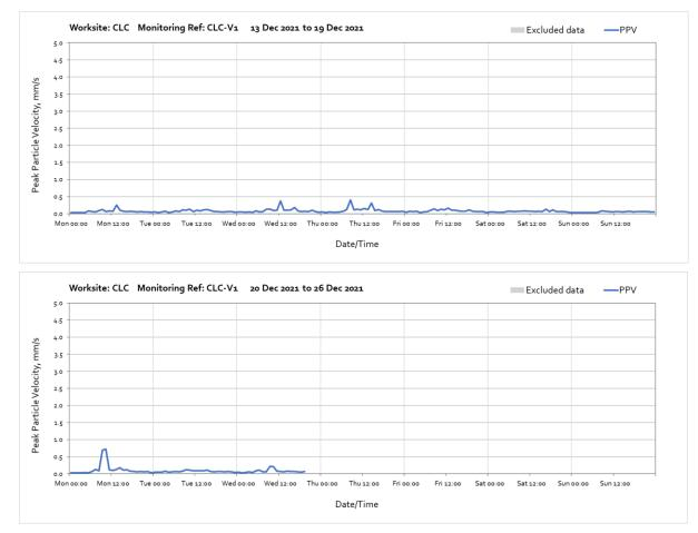
Note: Equipment power problems arising from weak sunlight caused the above missing data.
