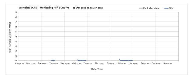
Note: Equipment power problems arising from weak sunlight caused the above missing data.
