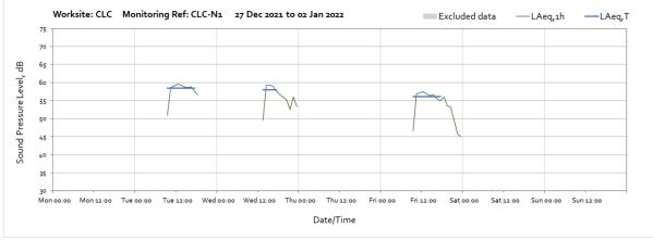
Note: Equipment power problems arising from weak sunlight caused the above missing data.
