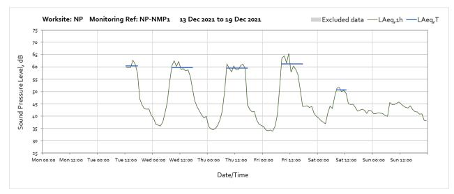
Note: Missing data from 21:00 on the 4<sup>th</sup> December until 12:00 on the 14<sup>th</sup> December was due to loss of power from external batteries. The monitor will have mains power to prevent loss of data in the future.
