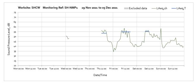
Note: Missing data between 04:00 on the 1<sup>st</sup> December until 12:00 on the 2<sup>nd</sup> December was due to loss of solar power because of lack of sunlight and no wind turbine power source. Wind turbine power source will be installed soon to prevent issue occuring again.
