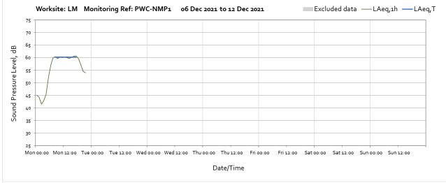
Note: Missing data from 22:00 on the 6<sup>th</sup> December till 19:00 on the 13<sup>th</sup> December was due to loss of power from external batteries. The monitor is expected to have mains power going forward.
