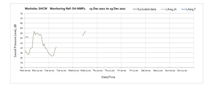
Note: Missing data between 08:00 on the 14<sup>th</sup> December until 09:00 on the 15<sup>th</sup> December was due to. loss of solar power because of lack of sunlight and no wind turbine power source. Wind turbine power source will be installed soon to prevent issue occuring again.
