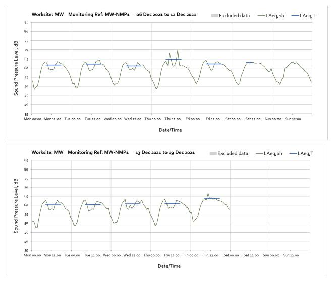
Note: Missing data from 00:00 on the 18<sup>th</sup> December till the end of December was due to technical issues from the charging controller. The battery and charge controller have now been replaced.
