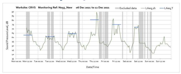
Note: N055\_New starts from 11:00 on Monday  $6^{th}$  December 2021 due to relocation from N055\_Old location. High noise level at 15:00 on Thursday  $9^{th}$  December 2021 was due to a flaw saw being used to install pipes within 3 metres of the monitor.
