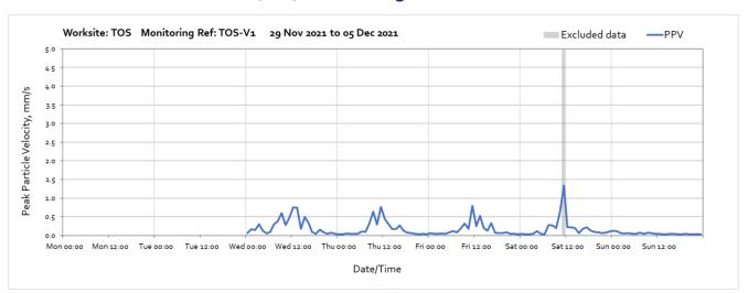
Note: Higher Vibration levels measured at 11:00 on Saturday 4<sup>th</sup> December was due to local inference with the monitor, which are not representative of HS2 construction works.
