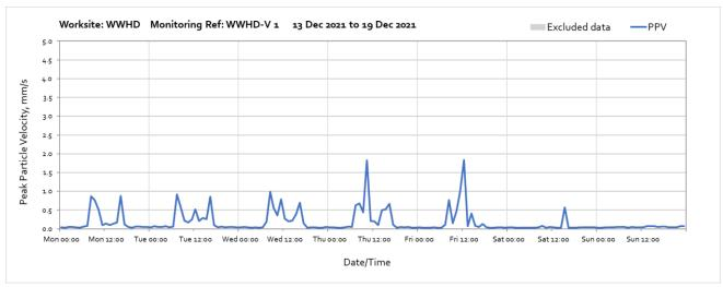
Note: Higher vibration levels measured during the week were due to plant working on north side of haul road, roller and dosser working and ground prep for unexploded ordinance (UXO) survey probing, and plant movement of a 30<sup>t</sup> excavator for removing concrete blocks in the area.
