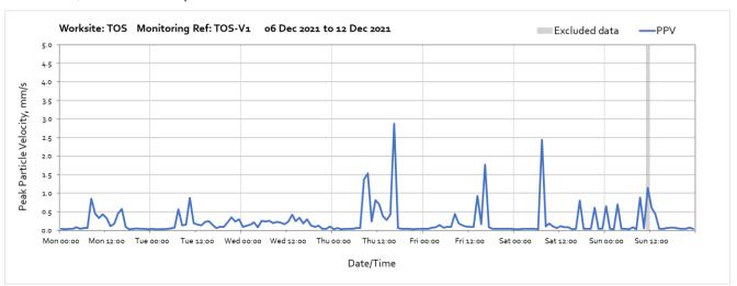
Note: Higer vibration levels measured across the week were due to installation of troughs, steel fixing, pouring of Slurry Treatment Plant (STP) slab, maintenance and operation of crane, and shuttering installation of precast troughs.
