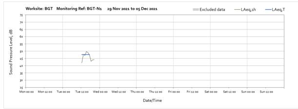
Note: Missing data throughout the week were due to loss of solar power to the equipment. To ensure there is no loss of power again batteries have been installed and are replaced frequently.
