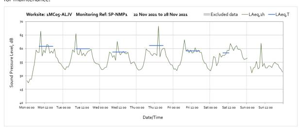
Note: Missing data between 01:00 and 02:00 on Sunday 28th November was due to loss of communication connection with the monitor.
