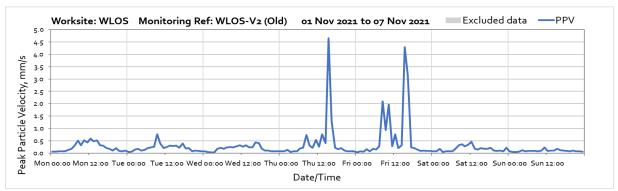
Note: Higher vibration levels are due to material haulage using HGV and backfilling/compacting of haul road that has been carried out on haul roads between Hodgetts Ln and Little Beanit Farm.
