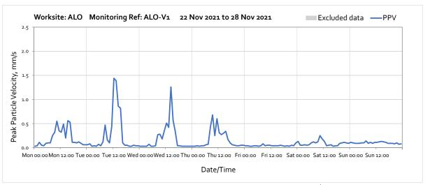
Note: High vibration levels measured in between 12:00 and 13:00 on Tuesday 23<sup>rd</sup> September 2021 were due to machinery in the area working for the construction of haul roads and moving stockpiles within the site. The nearest residential receptors are further away from the works and vibration levels at the receptors will therefore be lower.
