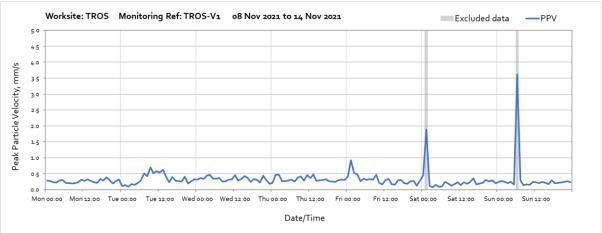
Note: The high vibration levels measured on Saturday and Sunday were due to local disturbance at the monitoring station were not representative of HS2 vibration level at the nearest receptor.
