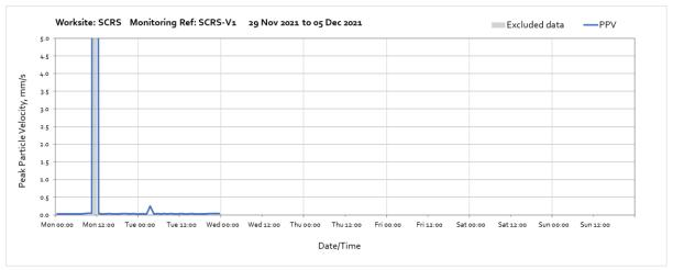
Note: The high vibration levels measured on Monday were due to local disturbance at the monitoring station and were not representative of HS2 vibration level at the nearest receptor.
