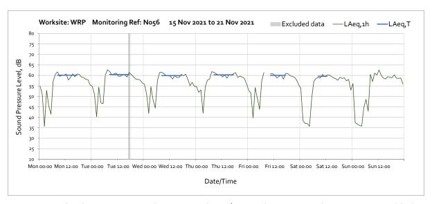
Note: Missing data between 08:00 and 10:00 on Friday  $19^{th}$  November 2021 was due to memory card fault at the monitoring station.
