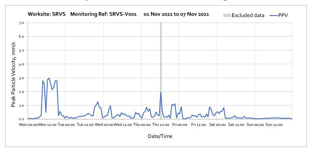
Note: High vibration levels measured in between 09:00 and 18:00 on Monday 1<sup>st</sup> November 2021 were due to the impact of the grab with concrete pilling platform.
