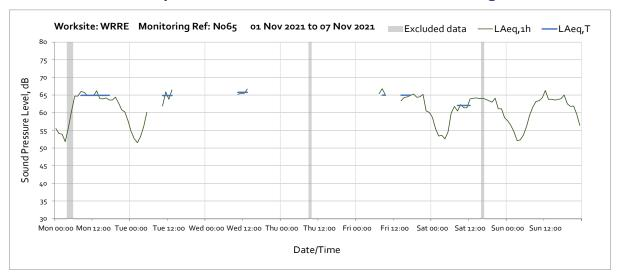
Note: Missing data throughout the week was due to loss of battery power at the monitoring station. OFFICIAL
