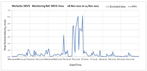
Note: High vibration levels measured across the week were due to the impact of the grab with concrete pilling platform therefore work methodology subsequently changed.
