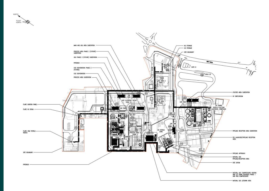
Figure 8.2<sup>22</sup> - HyNet Hydrogen Production Plants 1 and 2 Plot Plan.
