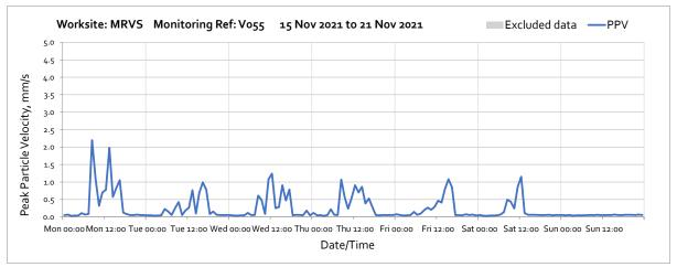
Note: High vibration levels measured across the week were caused by the access road maintanence works undertaken in proximity of the vibration monitor location.
