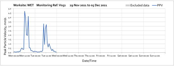
Note: High vibration levels measured from 12:00 until 16:00 on Monday 29<sup>th</sup> November and from 09:00 until 15:00 on Tuesday 30<sup>th</sup> November were due to concrete cutting using a floor saw.
