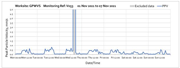
Note: High vibration levels measured in between 15:00 and 16:00 on Wednesday 3<sup>rd</sup> November 2021 were due to residents activity close to the vibration monitor and not representative of HS2 vibration levels.
