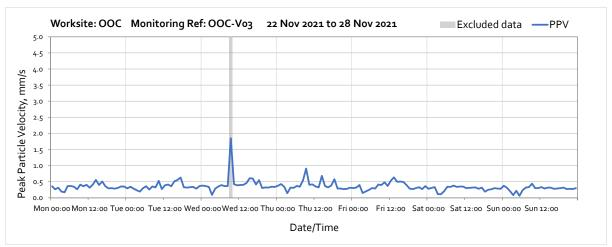
Note: High vibration levels measured at 09:00 on Wednesday 24<sup>th</sup> November were due local disturbace and not representative of HS2 vibration levels.
