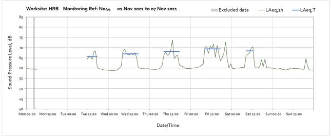
Note: Missing data from 07:00 on Monday 1<sup>st</sup> November until 11:00 on Tuesday 2<sup>nd</sup> November was due to a loss of power to the monitor. Continuous noise levels measured throughout the week were caused by an operational generator near to the monitor. The nearest receptor is located further from the generator and will therefore experience lower noise levels.
