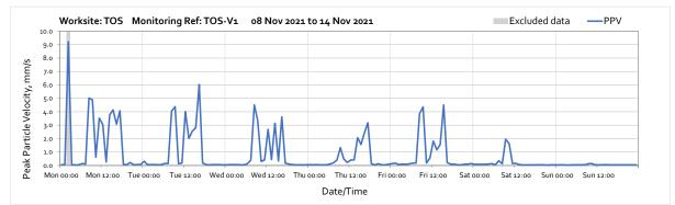
Note: High vibration levels across the week were due to backfiling and levelling work activites around the Slurry Treatment Plant (STP) platform area for the concrete blinding extension over duct runs taking place near to the monitoring equipment.
