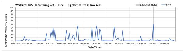
Note: High vibration levels across the week were due to backfiling and levelling work activites around the Slurry Treatment Plant (STP) platform area for the concrete blinding extension over duct runs taking place near to the monitoring equipment.
