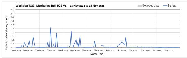
Note: High vibration levels across the week were due to backfiling and levelling work activites around the Slurry Treatment Plant (STP) platform area for the concrete blinding extension over duct runs taking place near to the monitoring equipment.
