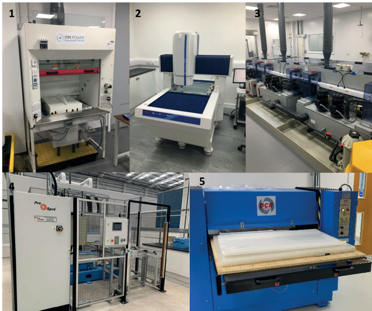
Figure 4-3: (1) Precious Metal Coating Electro-Deposition | (2) Visual Measurement Machine | (3) Precious Metal Coating Electro-Plating | (4) Robotic Welding Process | (5) Hot Press
