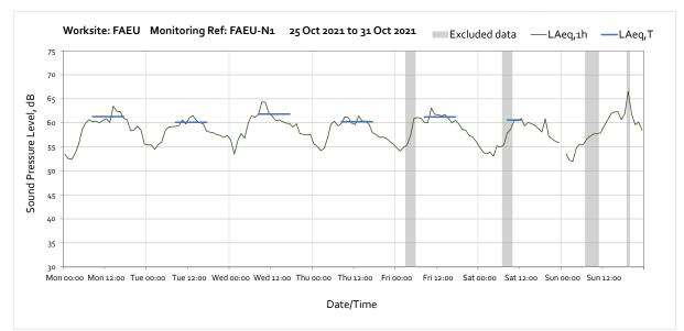
Note: Missing data between 00:00 and 01:00 on Sunday 31st October was due to sound level meter daylight saving time adjustment.
