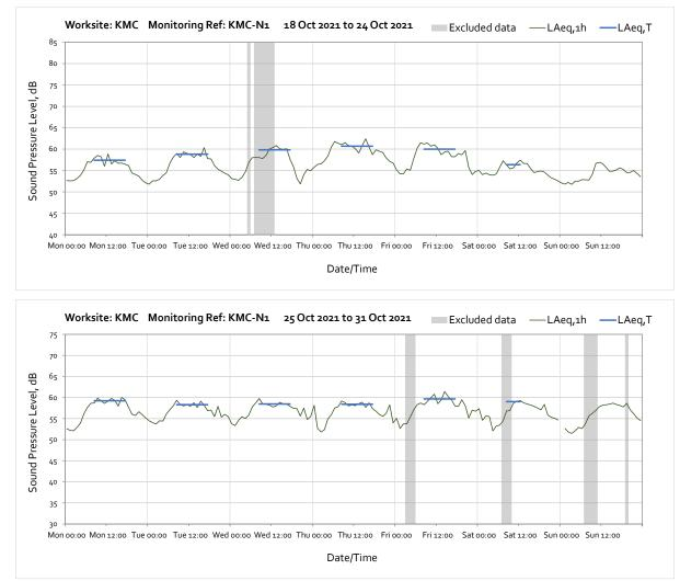
Note: Missing data between 00:00 and 01:00 on Sunday 31st October was due to sound level meter daylight saving time adjustment.
