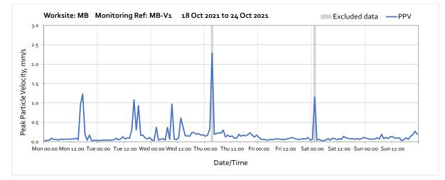
Note: High vibration levels measured in between 16:00 and 17:00 on Monday 18<sup>th</sup> October 2021 were due to continued excavation works, soil movement and digging works undertaken near to the monitoring location. The nearest residential receptors are further away from the works and vibration levels at the receptors will therefore be lower.
