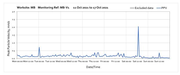
Note: High vibration levels measured in between 12:00 and 13:00 on Saturday 16<sup>th</sup> October 2021 were due to excavation works, soil movement and digging works undertaken near to the monitoring location. The nearest residential receptors are further away from the works and vibration levels at the receptors will therefore be lower.
