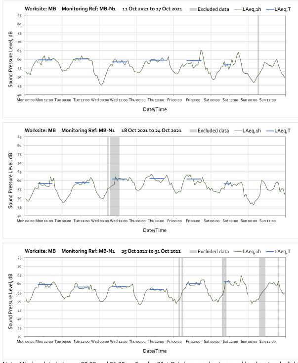
Note: Missing data between 00:00 and 01:00 on Sunday 31st October was due to sound level meter daylight saving time adjustment.
