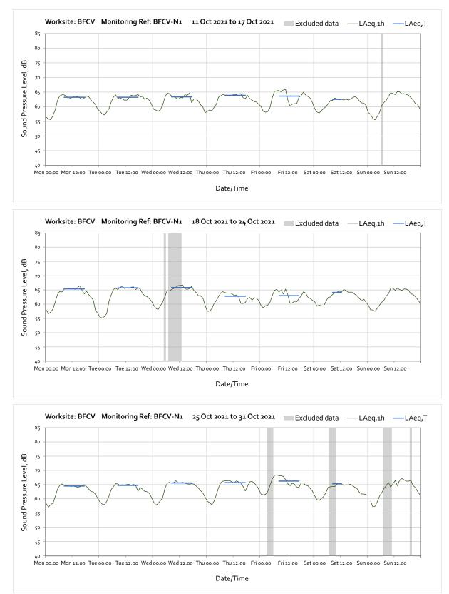
Note: Missing data between 00:00 and 01:00 on Sunday 31st October was due to sound level meter daylight saving time adjustment.
