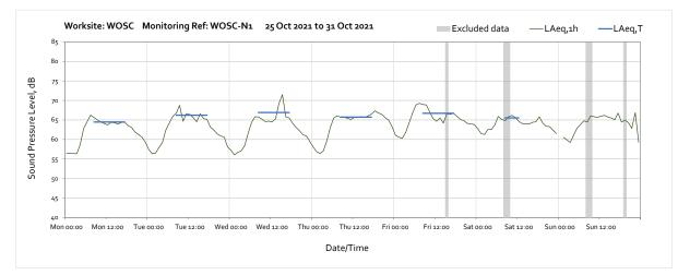
Note: Missing data between 00:00 and 01:00 on Sunday 31st October was due to sound level meter daylight saving time adjustment.
