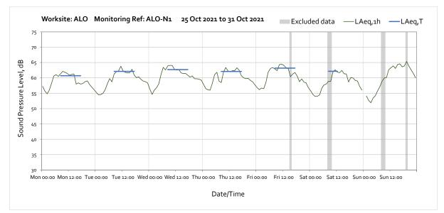
Note: Missing data between 00:00 and 01:00 on Sunday 31st October was due to sound level meter daylight saving time adjustment.
