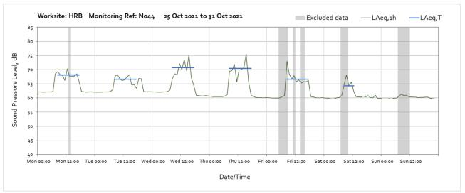
Note: Continuous noise levels measured throughout the week were caused by an operational generator near to the monitor. The nearest receptor is located further from the generator and will therefore experience lower noise levels.
