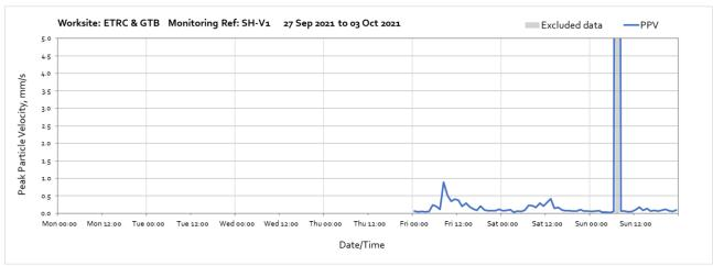
Note: High vibration levels measured at 07:00 on Sunday 3<sup>rd</sup> October were due to local interference of the monitor and are not representative of HS2 vibration levels at the receptor.
