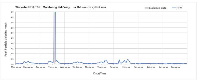
Note: High vibration levels measured at 14:00 on Tuesday 12<sup>th</sup> October were due to local interference of the monitor and are not representative of HS2 vibration levels at the receptor.
