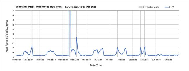
Note: High vibraton levels measured throughout the week were due to local interference of the monitor and are not representative of HS2 vibration levels at the receptor
