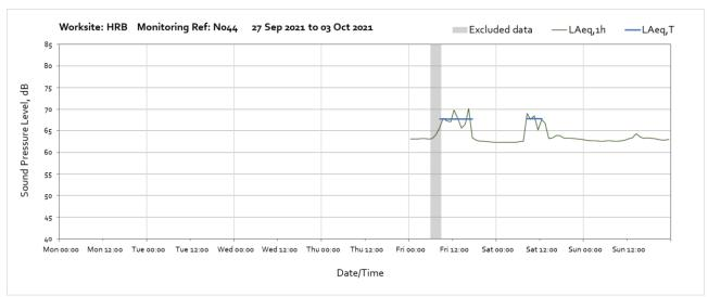
Note: Continuous noise levels measured throughout the week were caused by an operational generator near to the monitor. The nearest receptor is located further from the generator and will therefore experience lower noise levels.
