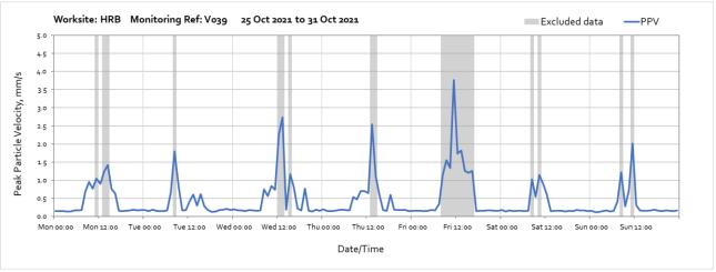
Note: High vibration levels measured throughout the week were due to local interference of the monitor and are not representative of HS2 vibration levels at the receptor
