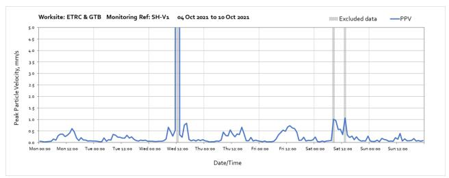
Note: High vibration levels measured throughout the week were due to local interference of the monitor and are not representative of HS2 vibration levels at the receptor.
