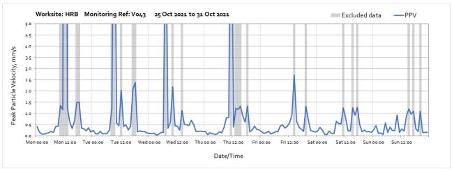
Note: High vibration levels measured throughout the week were due to local interference of the monitor and are not representative of HS2 vibration levels at the receptor.
