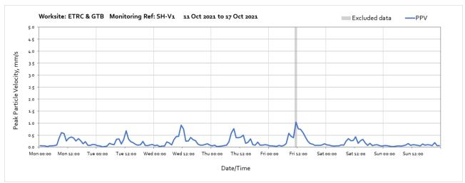
Note: High vibration levels measured at 11:00 on Friday 15<sup>th</sup> October were due to local interference of the monitor and are not representative of HS2 vibration levels at the receptor.
