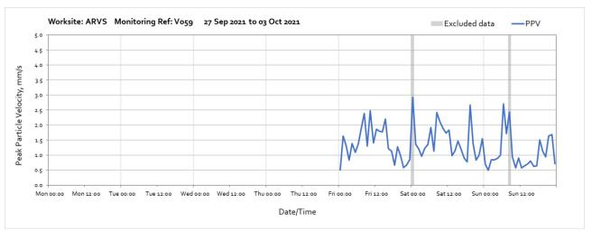
Note: High vibration levels measured at 00:00 on Saturday  $2^{nd}$  Ocobter and at 08:00 on Sunday  $3^{rd}$  October were due to local interference of the monitor and are not representative of HS2 vibration levels at the receptor.
