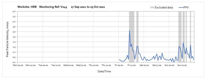
Note: High vibraton levels measured throughout the week were due to local interference of the monitor and are not representative of HS2 vibration levels at the receptor.
