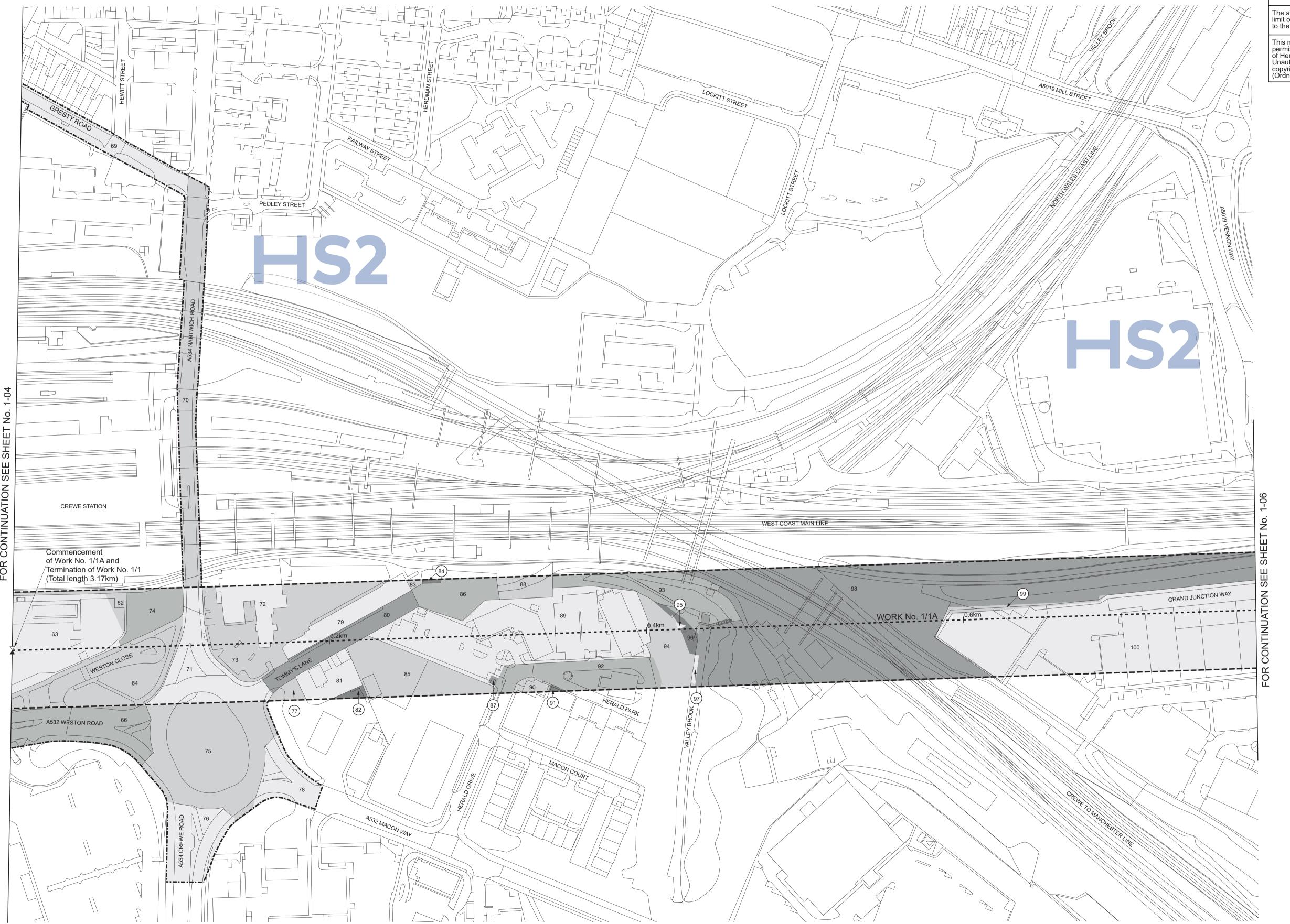
Proposed Tunnel below Valley Brook, Work No. 1/1A, depth of Tunnel below river bed 25.50m.
